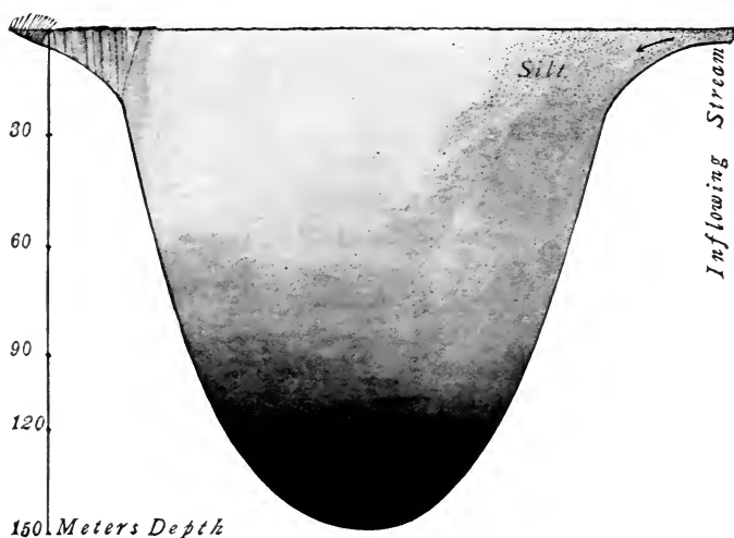
FIG. 3. Diagram illustrating the penetration of light into the water of a lake; also, its occlusion by inflowing silt and by growths of plants on the surface.
