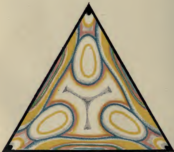
ISOCHROMATIC LINES IN A TRIANGLE OF UNANNEALED GLASS.
