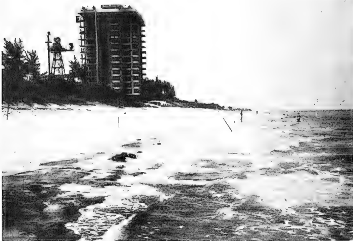
Figure 5. View north at Boca Raton site, 4 May 1970; low tide ( H = 1.0 ft; T = 4.6 s; \alpha_b = -20^\circ ). Note coquina exposure in swash zone.
