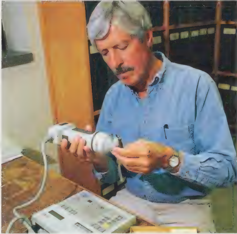
Ned Johnson, above, uses a reflectance spectrophotometer to determine the exact feather color of a specimen.
