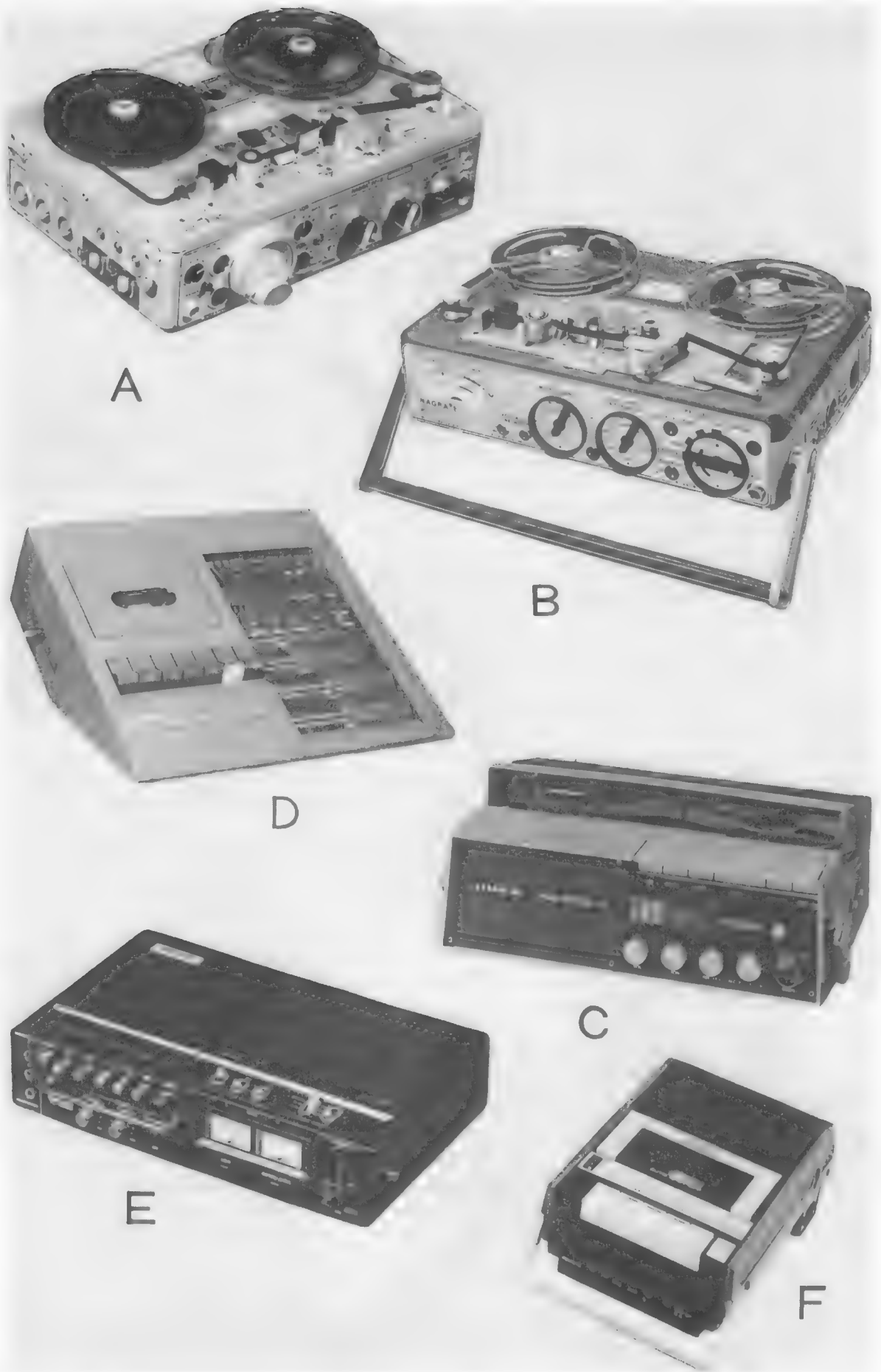
Figure 2. Representative tape recorders showing examples of available equipment in different price categories: A, Nagra IV-S; B, Nagra E; C, Yamaha 800GL; D, Uher 4000 IC; E, Sony TC153SD; F, Superscope C-101A.
