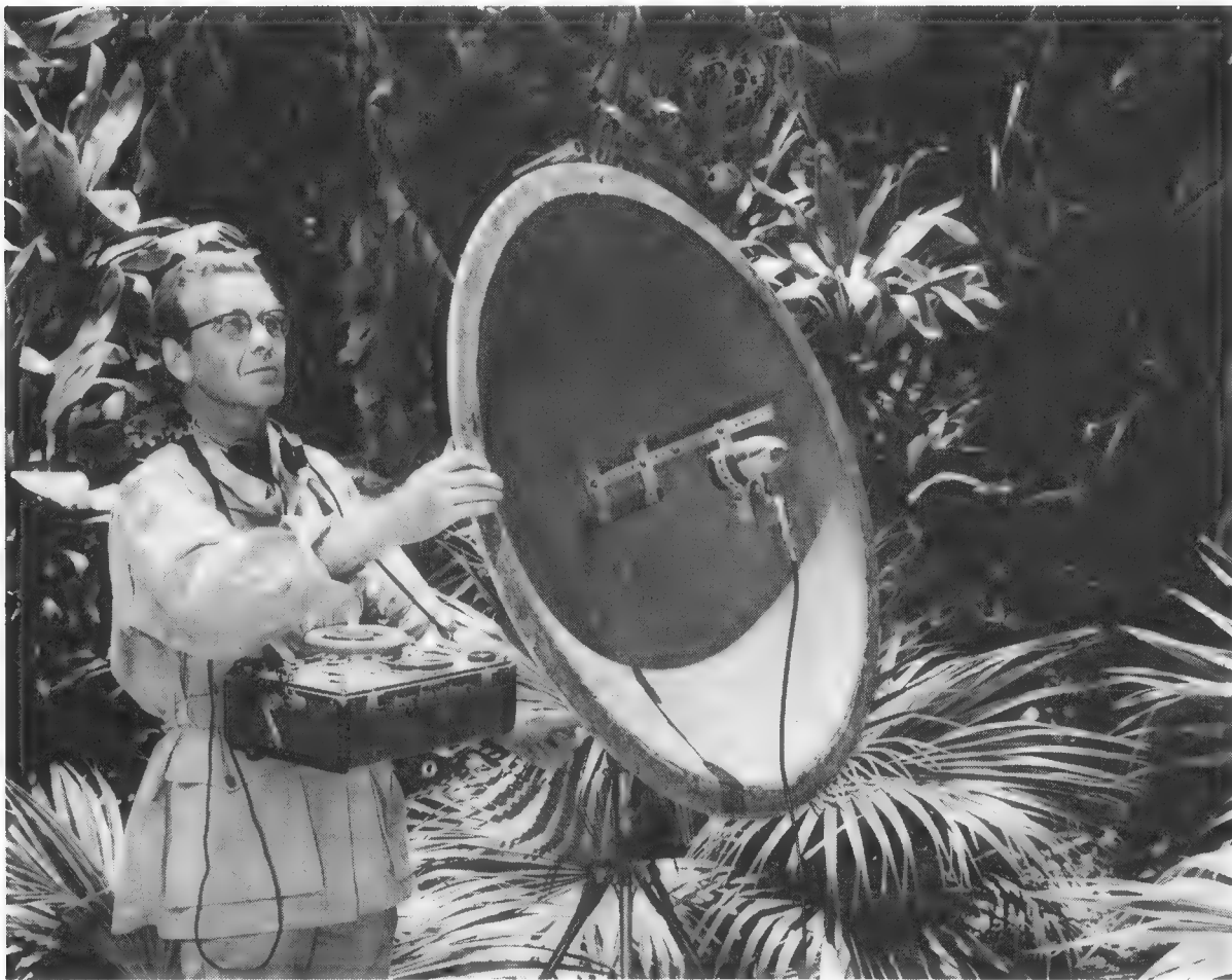
Above , Mr. Paul Schwartz, Research Associate of the Laboratory of Ornithology, recording bird voices in Venezuela with a Magnemite. The reflector was supplied by Dr. William W. H. Gunn of Toronto, Canada.
