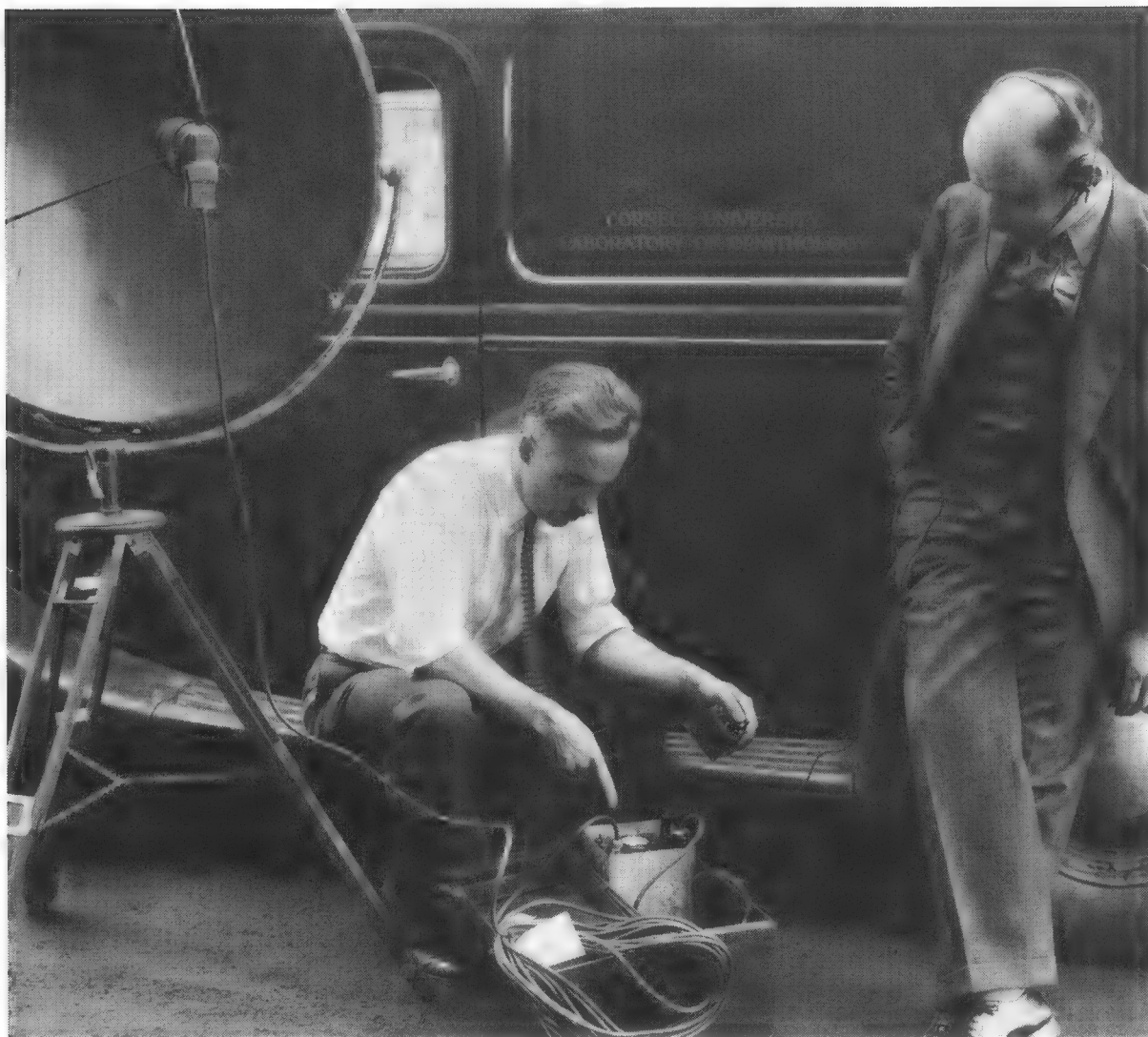
The author shows Albert R. Brand (right) a new battery-operated preamplifier which enabled weak microphone signals to be increased so that they could be transmitted over an open wire line to the sound truck (in background) several miles away. Photograph taken in 1937 by Arthur A. Allen.
