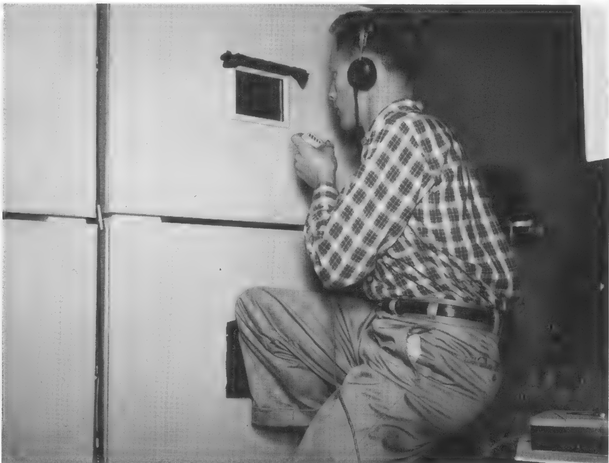
Figure 2. Hartshorne Sound Isolation Chambers, showing method of observation (through "one-way glass"), sound monitoring, and recording of data.
