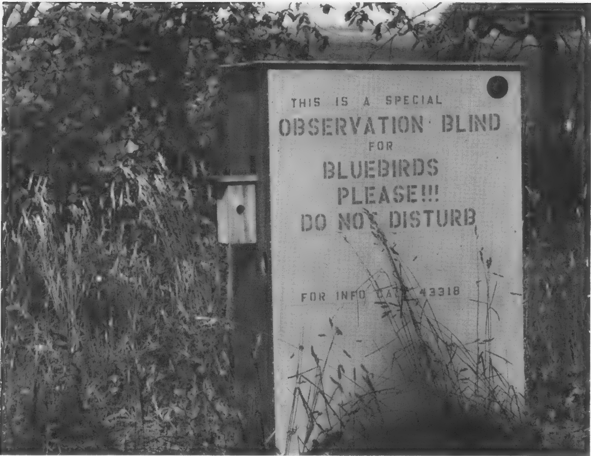
Figure 1. Special field nest box and blind used to obtain behavioral data at a Bluebird's nest. Circular holes provide ventilation for the interior of the blind and connect with internal light baffles. Square hole in the blind over the nest box contains "one-way glass," which permits observing the behavior of birds on the roof of the nest box.
