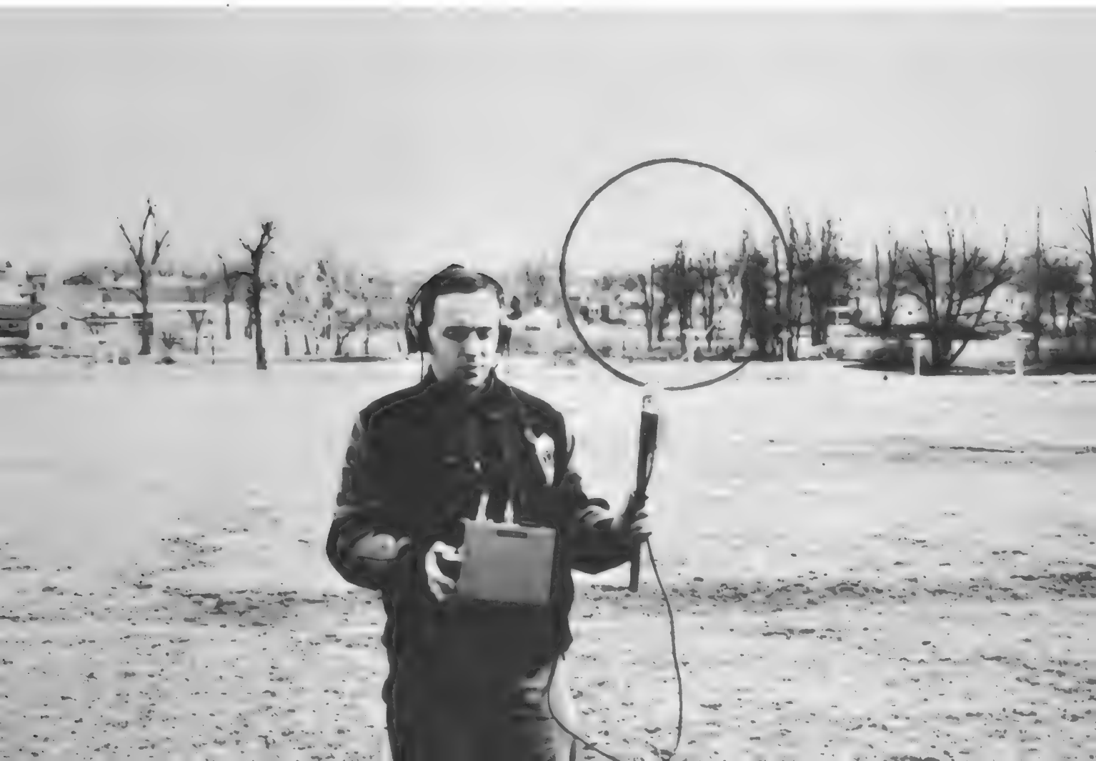
Figure 5 (below). A transistorized tracking receiver being used as a portable unit. Note the hand-held loop antenna and the headphones.
