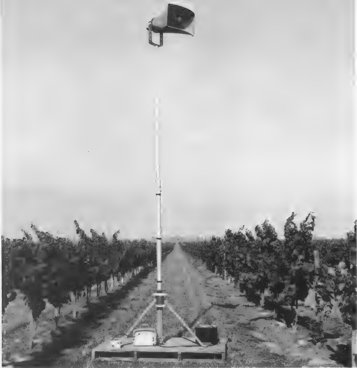
Figure 3. An automatic sound source in a vineyard. Sound projections are scheduled by an electronic programmer. The speaker rotates during the sound emissions and effectively covers an area 2,000 feet in diameter.
