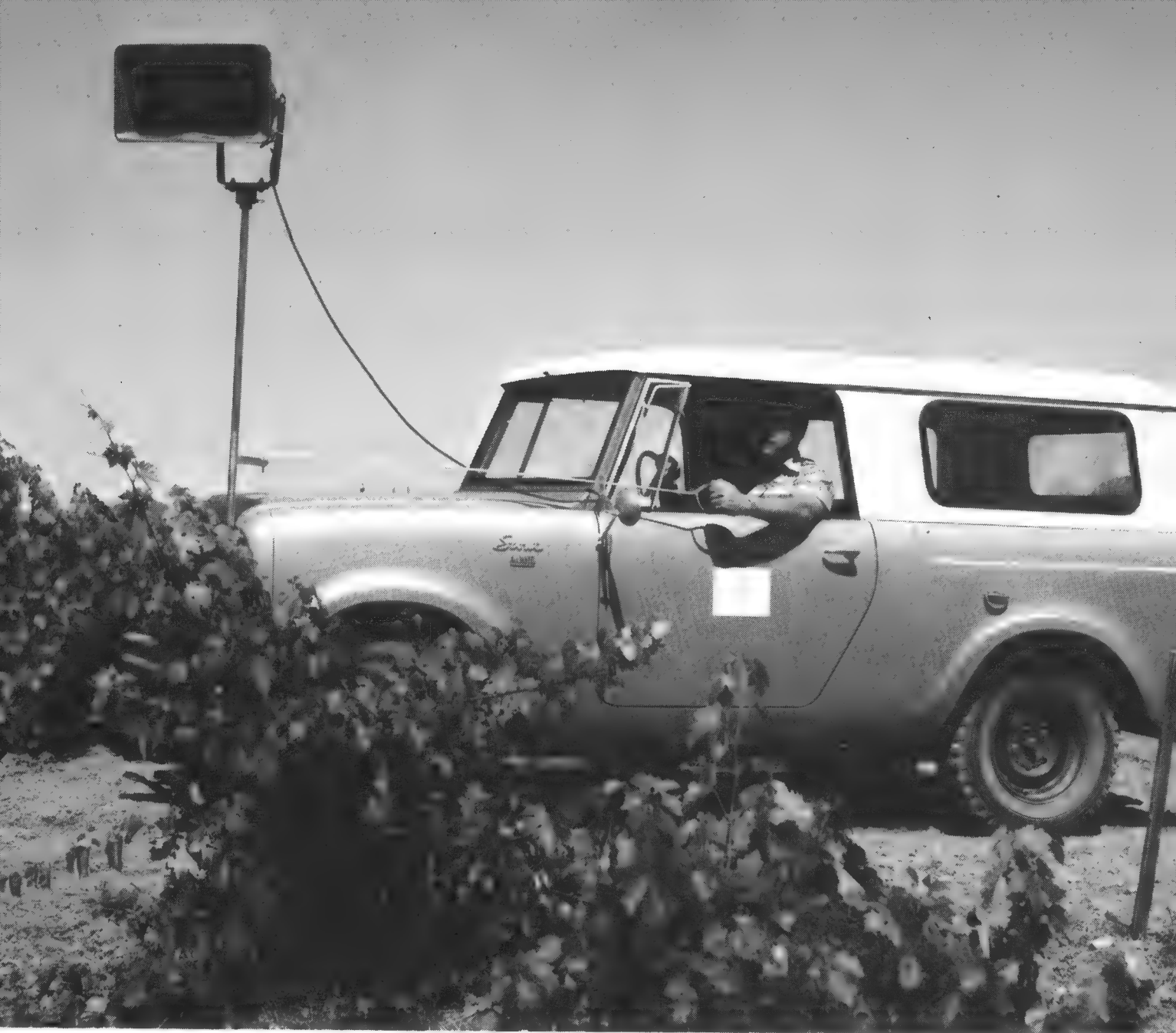
Figure 2. Experimental sounds being evaluated in a vineyard. The operator remains in the vehicle and manually regulates the sound and aims the loudspeaker.
