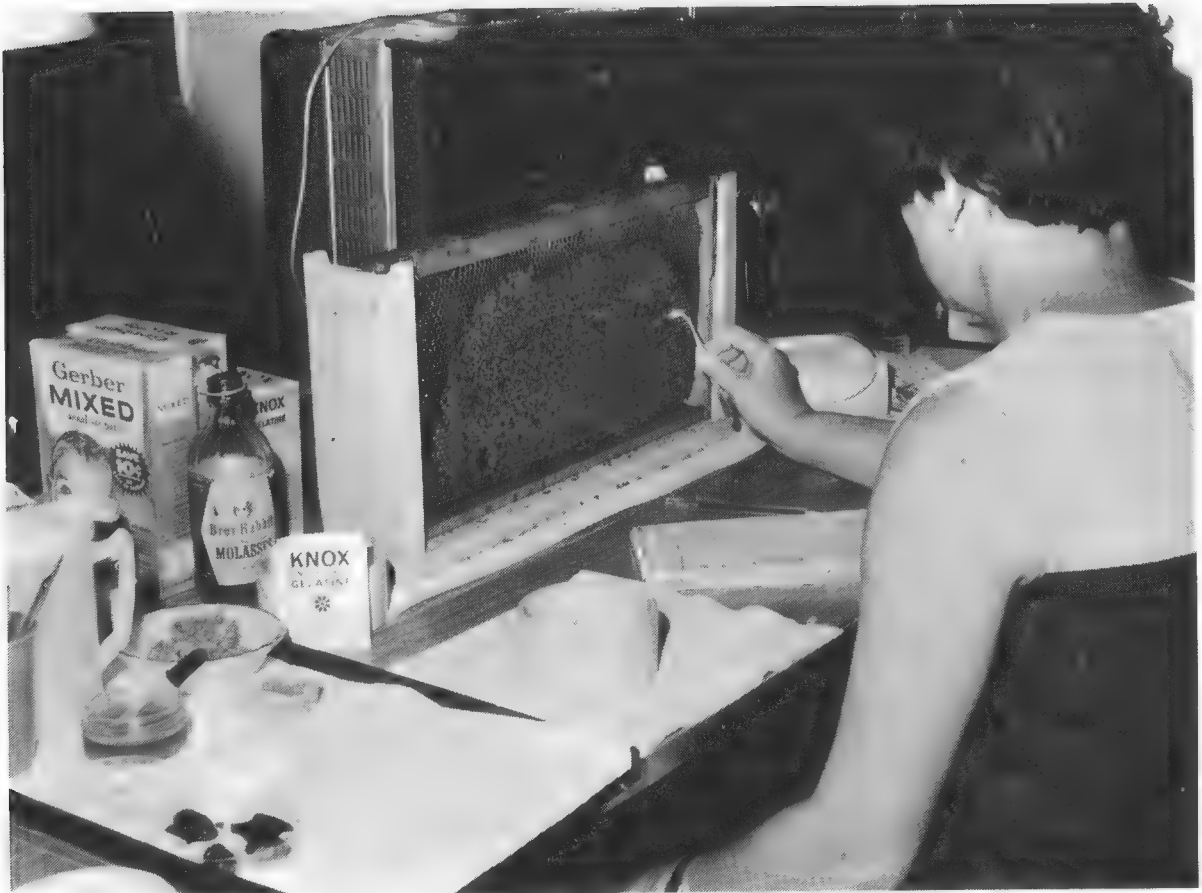
Figure 6. A frame containing honey bee brood of assorted ages is brought into the laboratory where the dietary mixtures are prepared. The capped cells are opened easily with forceps and the pupae extracted as needed.
