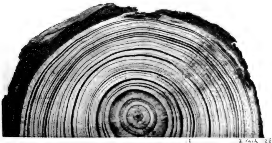
B. Wood from tree growing on very wet soil, showing characteristic irregularity of grain. (Author's illustration.)
