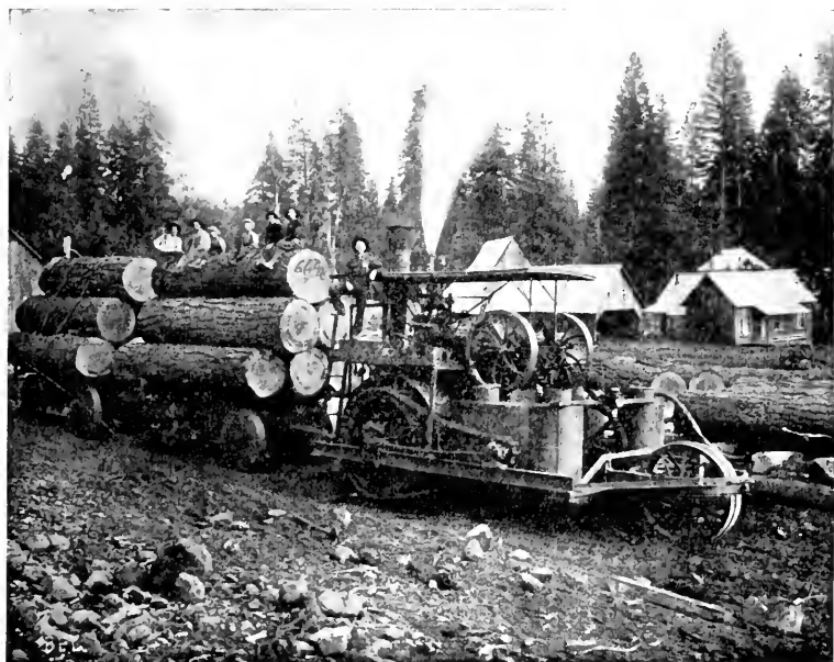
FIG. 58. — A Holt Three-wheeled Traction Engine hauling Sugar Pine Logs. California.
