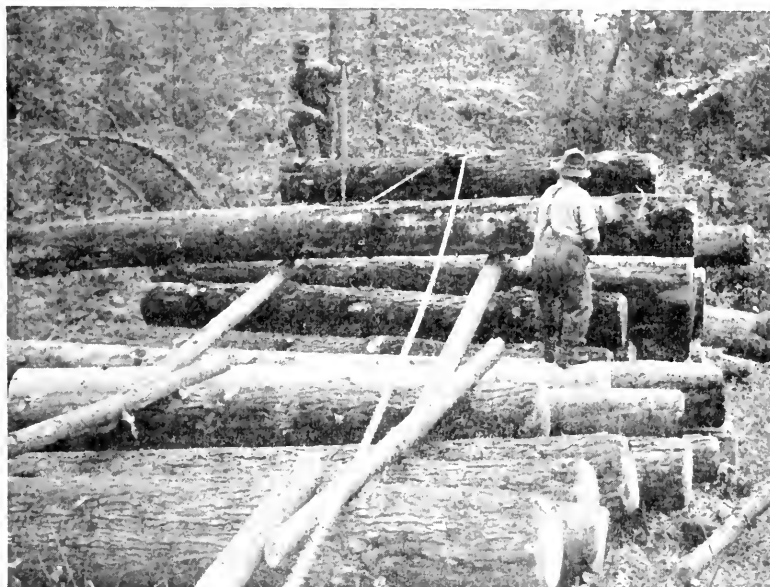
FIG. 24. — Decking Logs with a Crosshaul, the Block being fastened at the Front End of the Skidway. New York.
