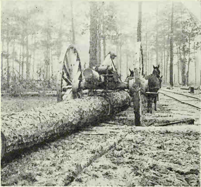
FIG. 54. — A Two-wheeled Slip-Tongue Log Cart hauling Long Logs. Note the rotating bunk above the cart axle, to which the grab chains are attached. Texas.
