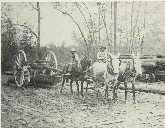
FIG. 53. — A Slip-tongue Log Cart, showing the Position of the Load during Transit. The short lever arm above the main tongue is attached to the rotating bunk to which the timber grabs are fastened. It automatically assumes a nearly vertical position, when the cart tongue is pushed to the rear. Texas.
