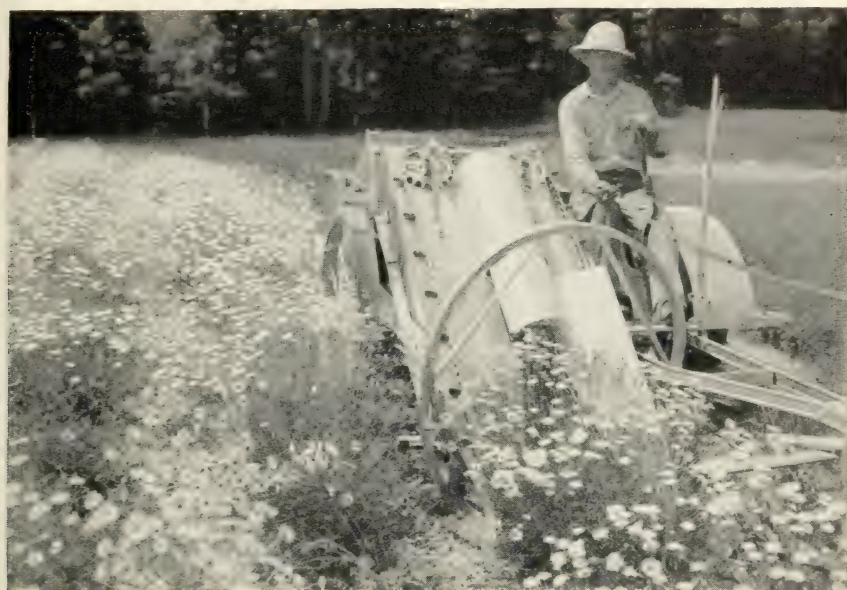
FIGURE 16.—Mechanical pyrethrum picker developed by U. S. Department of Agriculture.
