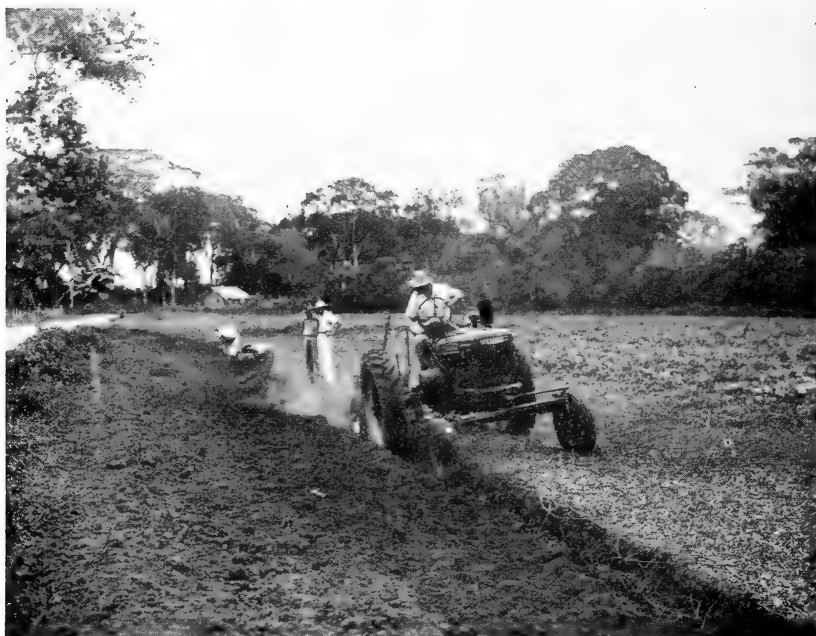
FIGURE 14.—Whirlwind terracer being used in derris harvest trials for digging roots after tops were removed with other equipment. Tractor was operated in low gear and terracer in low speed.
