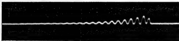
FIG. 8.—Oscillations with primary of magneto closed.
