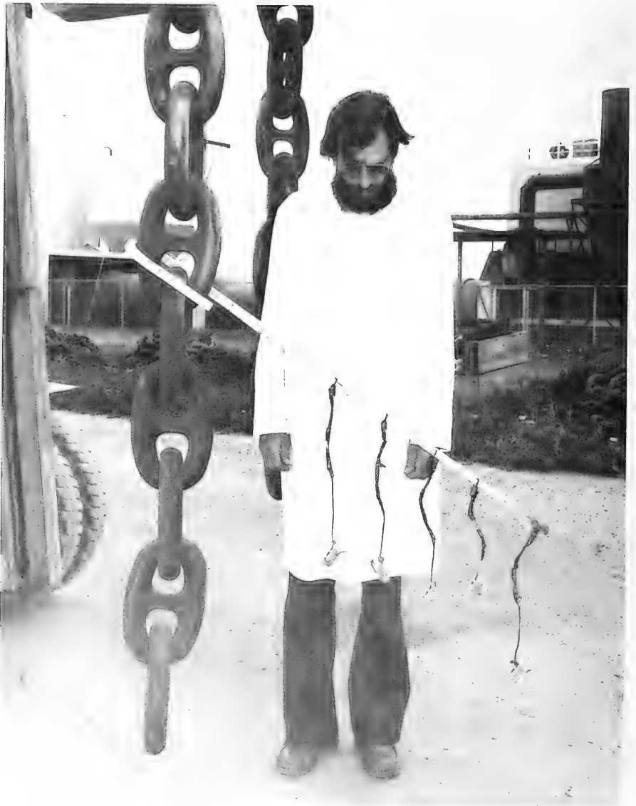
Figure D-1. Arrangement for suspending cement samples from chain of Spheres no. 15 and 16.
