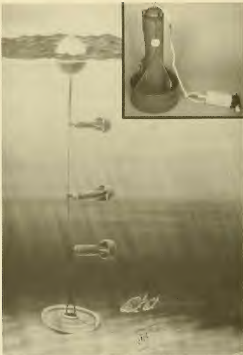
Figure 6. In situ current meter (inset) and typical current meter mooring string
