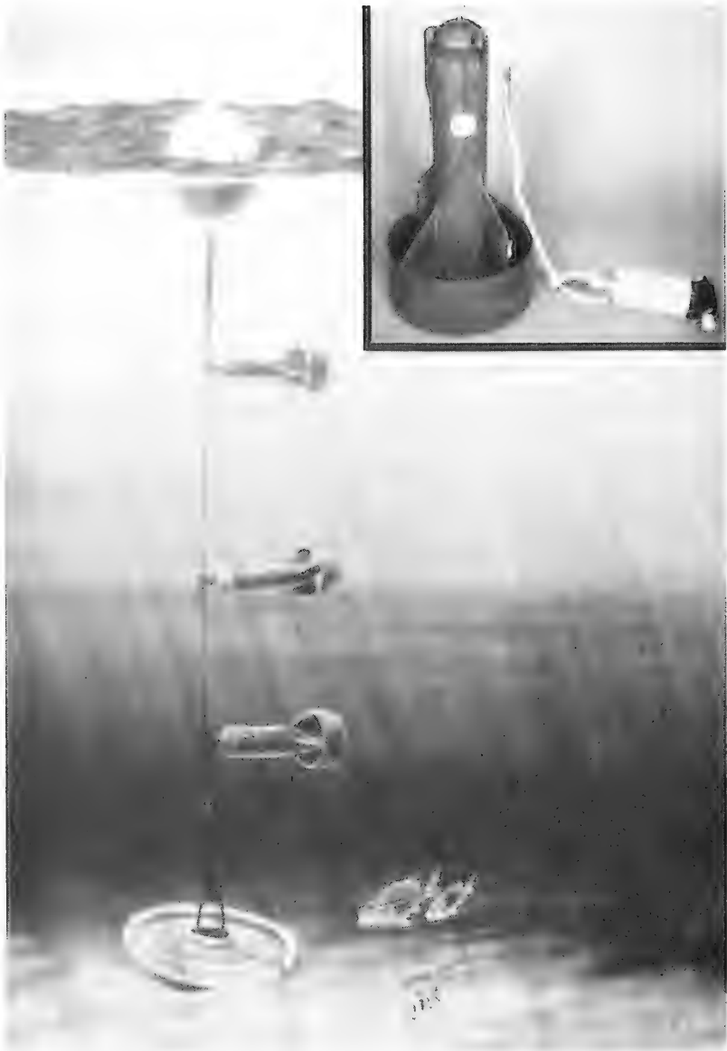
Figure 6. In situ current meter (inset) and typical current meter mooring string
