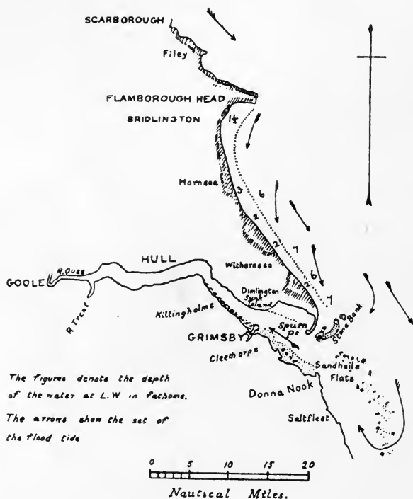
MAP SHOWING THE DIRECTION OF THE CURRENTS WHICH BRING THE MUD DOWN THE COAST AND INTO THE HUMBER.
