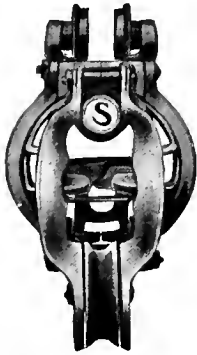
Cut A The end of the rope is fastened in the Carrier with our patent swivel iron knot, as shown in A. The rope is placed through the tilting eye, S (Fig. C 430), and the iron knot resting loosely thereon makes a complete, durable and simple swivel, which lets all kink and twist out of the rope.
