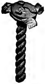
Cut A The end of the rope is fastened in the Carrier with our patent swivel iron knot, as shown in A. The rope is placed through the tilting eye, S (Fig. C 430), and the iron knot resting loosely thereon makes a complete, durable and simple swivel, which lets all kink and twist out of the rope.
