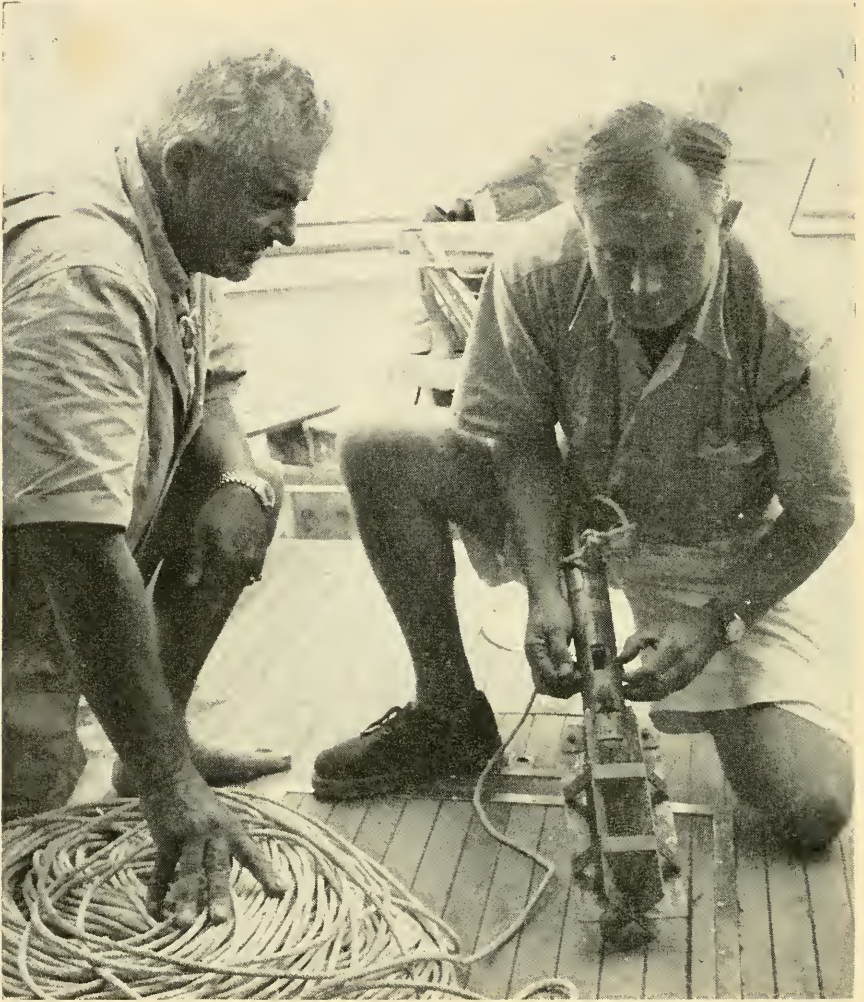
FIGURE 7. Mr. Lou Marron and Dr. F. G. Walton Smith, setting bathythermograph for recording of subsurface temperatures off the coast of Ecuador.
