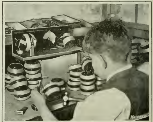
Fig. 4. Straightening the Shaft of a Variometer Rotor
