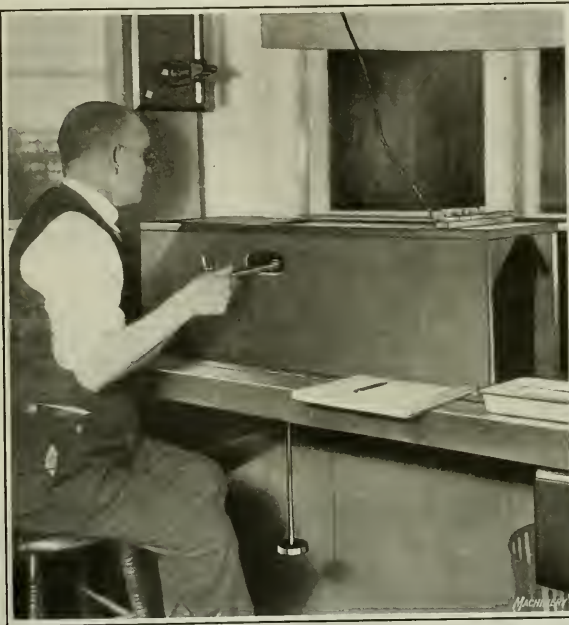
Fig. 8. View showing Case in which Comparator is enclosed when in Use to prevent Errors due to Temperature of the Observer's Body
