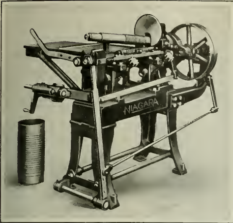
Fig. 2. Machine used to roll the Corrugated Sheet into the Form of a Pipe
