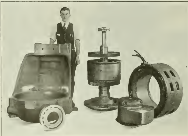
Fig. 3. Principal Parts of the Wheel-head
