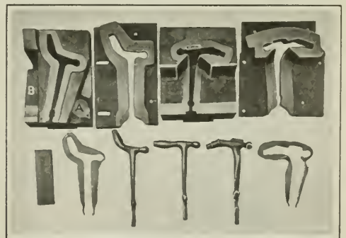
Fig. 7. Forging and Trimming Dies for Automobile Steering Arm
