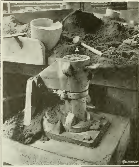
Fig. 2. Jolting Machine with Cast-iron Core-box in which the Core is jolted
