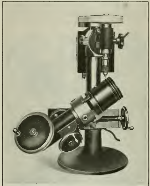
Fig. 2. Machine set up for Drilling Operation, the Work-spindle being at an Angle and the Upper Spindle Vertical
