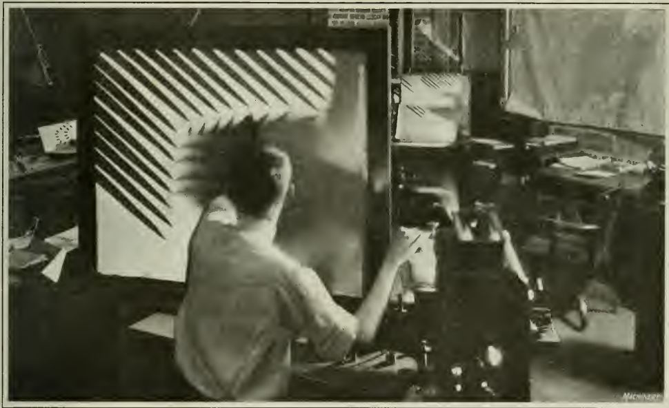
Fig. 1. Testing Outline of a Gear Tooth, the Image of which is reflected against the Mirror seen in the Background and then forward to a Ground Glass Screen at the Operator's Position
