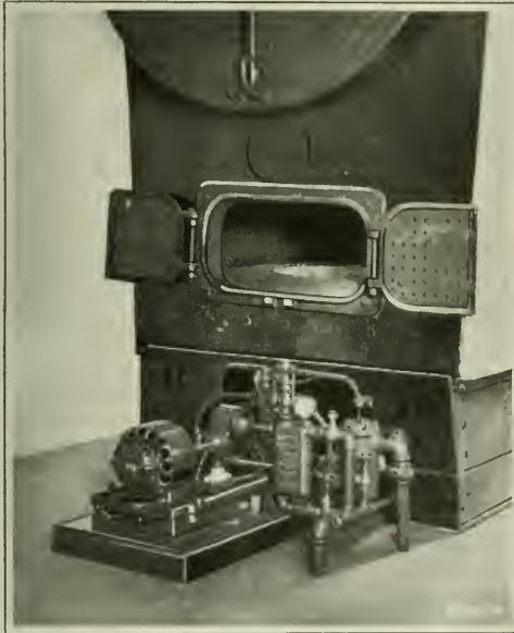
Fig. 1. Hardinge Oil Burner applied to Boiler
