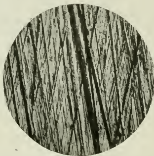
Fig. 2. Hand-lapped Plug Gage
