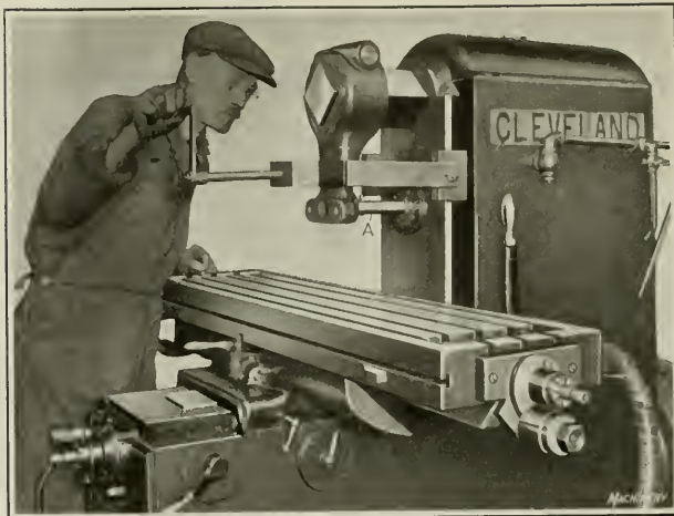
Fig. 5. Boring the Arbor Support Hole in the Over-arm Pendant
