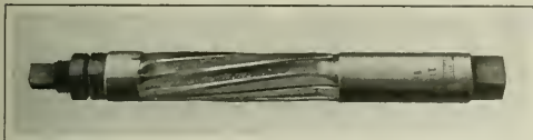
Hand Reamer of the Helical-flute Expansion Type made by the Pratt & Whitney Co.
