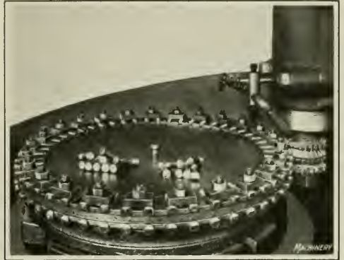
Fig. 2. Fixture for holding One Hundred Connecting-rod Bolts on a Single-spindle Machine
