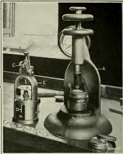
Fig. 1. Presses on which Watch Jewels and Bushings are staked in the Plates
