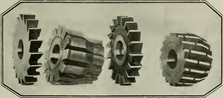
Formed Cutters used in Roughing and Finishing a Small Machine Part on a Brown & Sharpe No. 21 Automatic Milling Machine.
