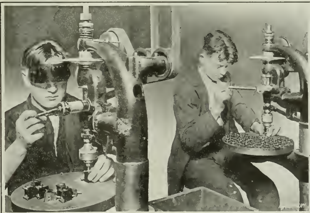
Fig. 8. Two Different Tapping Operations required on Radio Parts
