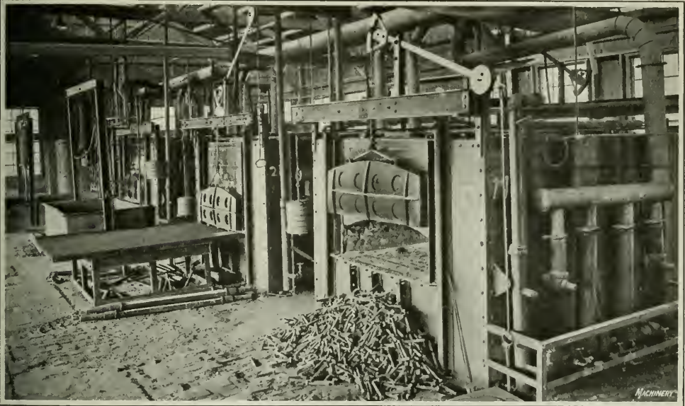
Fig. 2. Battery of Heat-treating Furnaces for Drop-forgings
