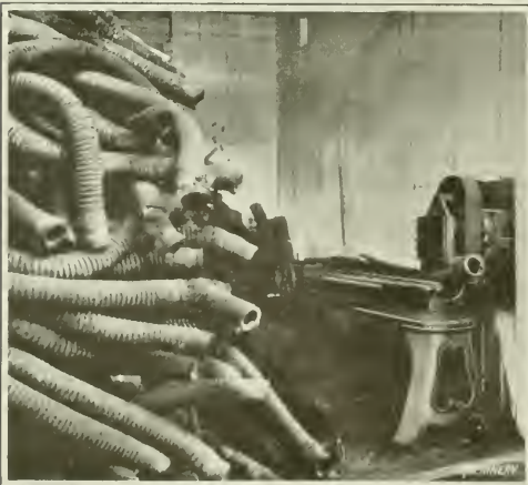
Fig. 2. Slitting Armored Rubber Steam Hose preparatory to removing the Wire
