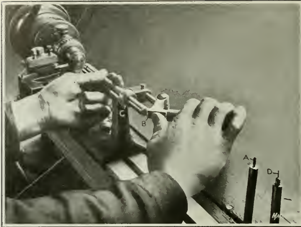
Fig. 5. Drilling the Hole in a Small Stud preparatory to tapping
