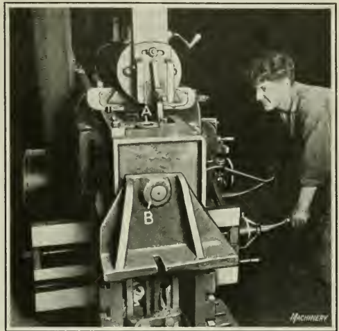
Fig. 9. Using an Indexing Shaper Fixture for planing Gear-boxes
