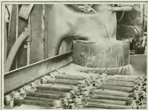
Fig. 6. Grinding the Side Faces of Connecting-rods
