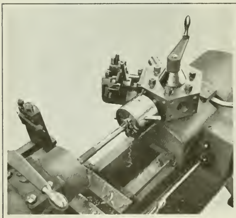
Fig. 2. Threading a Staybolt on the Lassiter-Milholland Model A Machine
