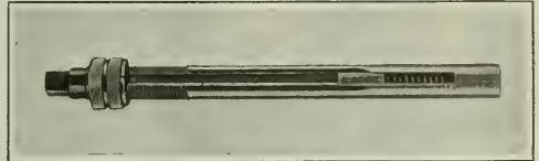
Tool for reaming Bushings of Automobile Pistons which is made by the Standard Tool & Supply Co.
