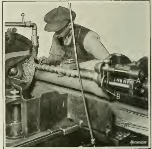
Fig. 12. Rear View of Grinding Machine showing Mechanism which controls the Cam-grinding Operation
