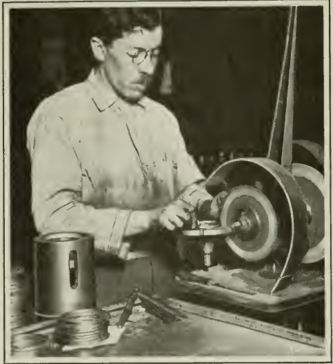
Fig. 2. Grinding Ends of Lap Joint before gaging for Expansion
