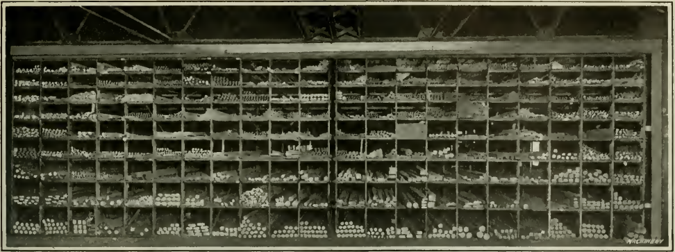
Fig. 4. Horizontal Storage Rack in which Special Grades of Drop-forging Steel are stored
