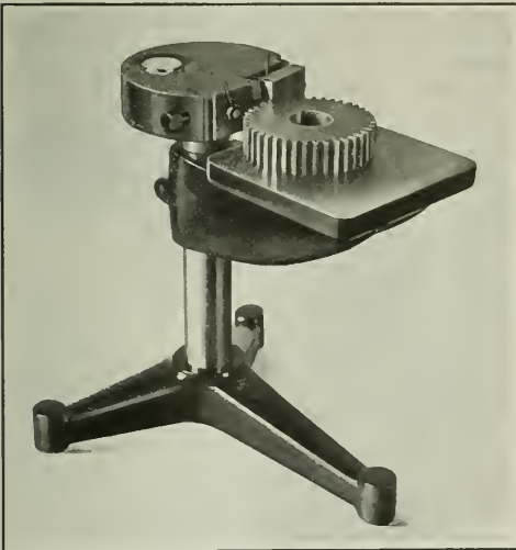
Fig. 2. Odontometer for Gears from 10 to 24 Diametral Pitch
