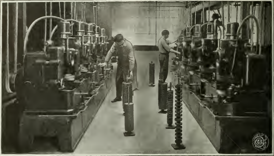
Battery Installation of New High-speed Gear Shapers. One 6-H.P. Motor furnishes Ample Power for Ten Machines.
