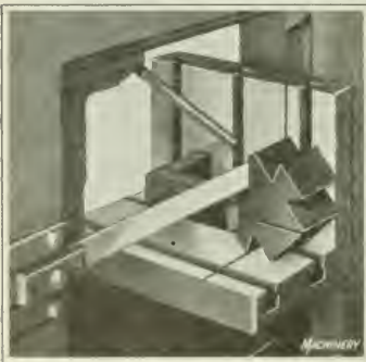
Fig. 4. Cutting Angular External Surfaces
