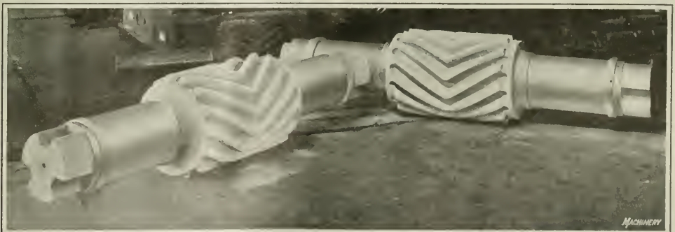
Fig. 1. Semi-shrouded Rolling Mill Herringbone Pinions machined by end-milling
