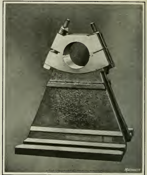
Fig. 13. Saddle for Dredge, showing Hole bored on Machine illustrated in Fig. 15
