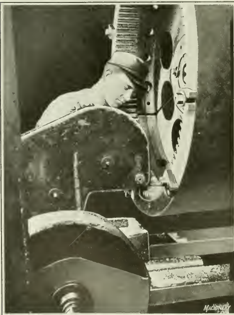
Fig. 2. Detail View of an Internal Gear-cutting Attachment at Work
