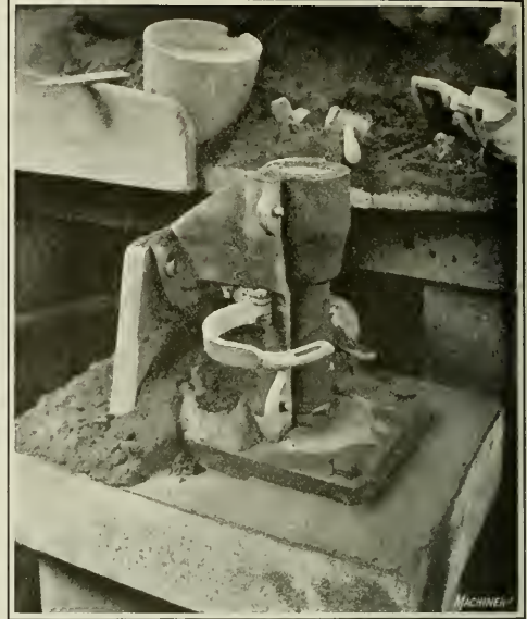
Fig. 3. Jolting Machine shown in Fig. 2, with Front Cover of Core-box removed
