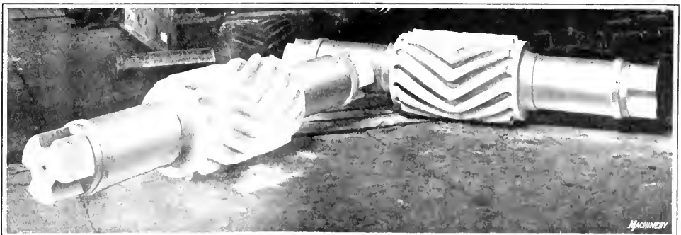
Fig. 1. Semi-hobbed Rolling Mill Herringbone Pinions machined by end-milling
