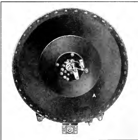
Fig. 19. Fixture for testing the Spacing of Lobes on Ignition Distributor Timing Cams
