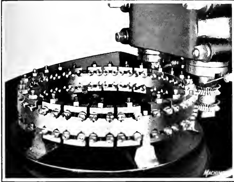
Fig. 1. Operation in which One End of Camshaft Thrust Blocks is flattened and beveled
