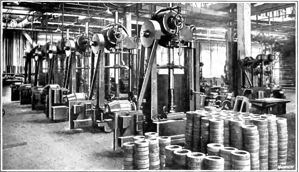
Fig. 1. Battery of Power Forcing Presses used in broaching Motor Stators
