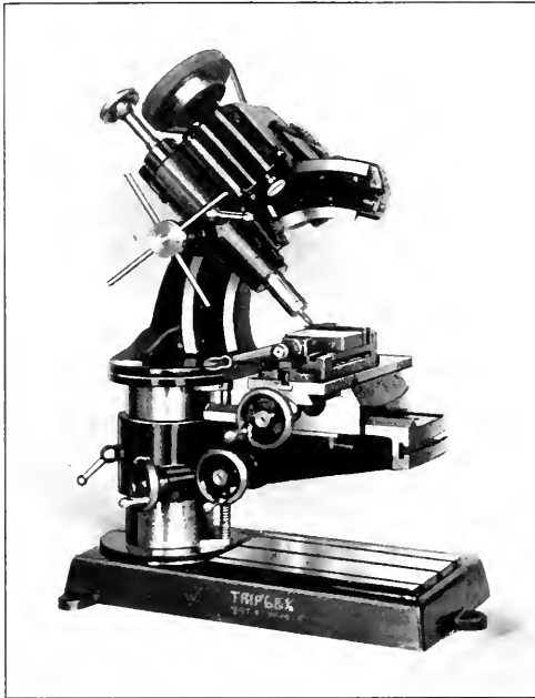
Fig. 2. Performing an End-milling Operation with the Spindle in an Angular Position
