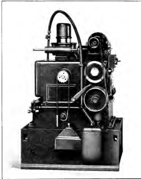
Fig. 2. Rear View of the Fellows High-speed Gear Shaper equipped with Individual Motor Drive
