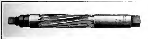
Hand Reamer of the Helical-flute Expansion Type made by the Pratt & Whitney Co.
