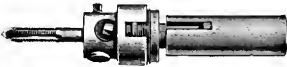
Interchangeable Spring Sheeks for Rough and Finish Taps occupying One Turret Hole.
