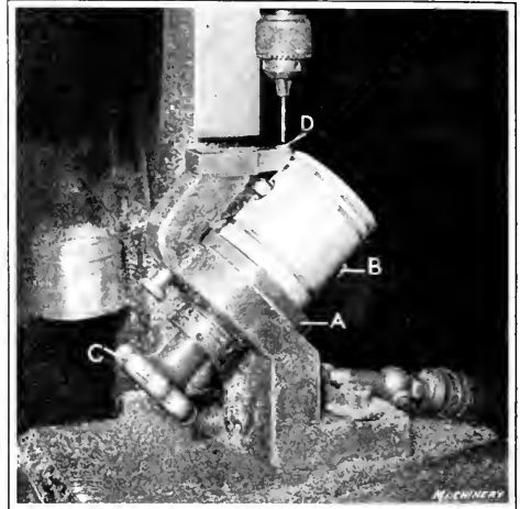
Fig. 7. Jig for drilling Two Inclined Oil-holes leading to Wrist-pin Bearings
