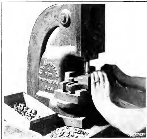
Fig. 5. Assembling the Fiber Flanges, using a Foot Press
