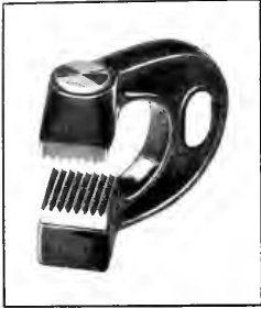
Fig. 1. New Type Thread Gage with U. S. Form of Thread
