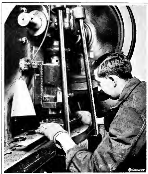
Fig. 6. Power Press equipped with Simple Stamping Dies for making the End Plates of Variable Condensers
