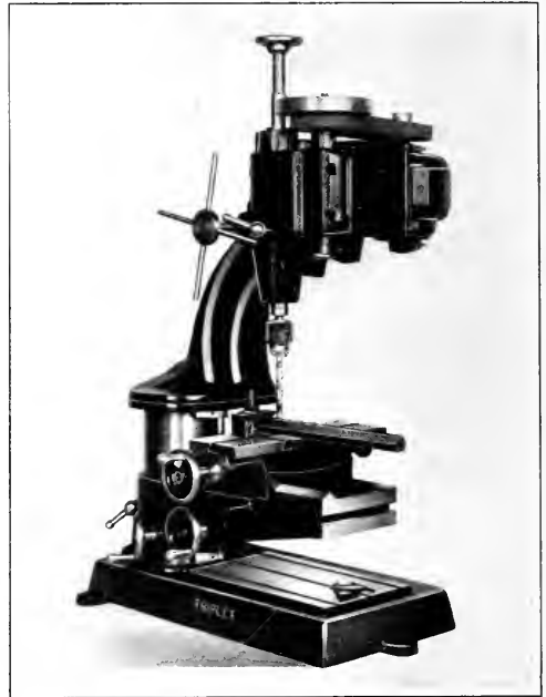
Fig. 3. A Drilling Operation in which the Spindle is placed in a Vertical Position
