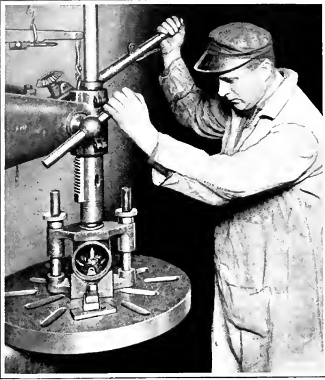
Fig. 5. Drilling Machine and Fixture used for holding Pistons while facing the Wrist-pin Bosses
