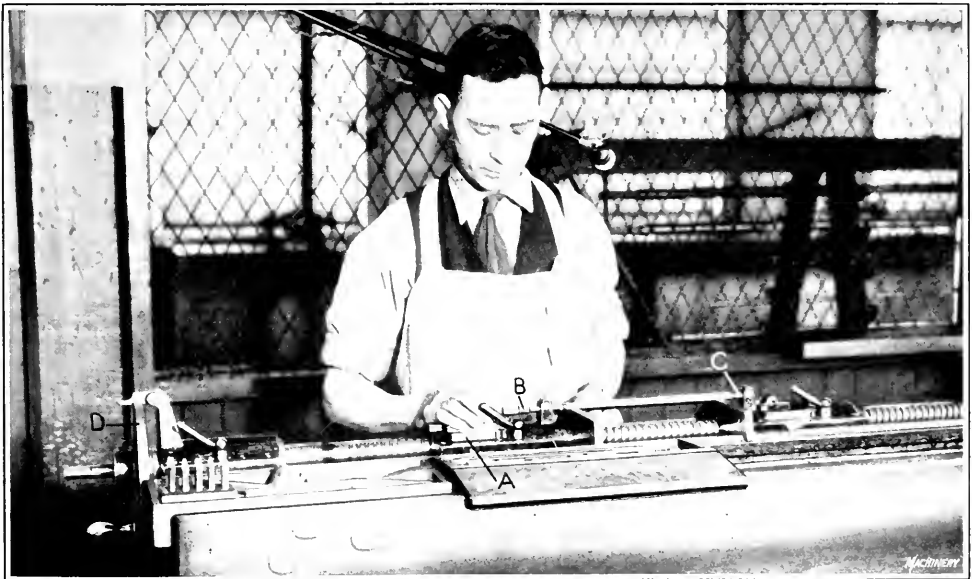
Fig. 2. Standard End-measuring Gage inserted between Anvil and Micrometer Spindle to show Lead Errors
