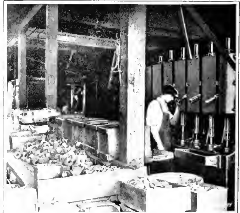
Fig. 3. Multiple-spindle Nut-tapping Machine used for rethreading Old Nuts
