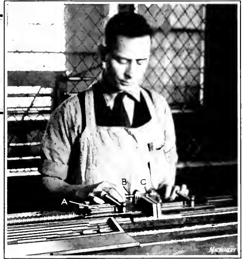
Fig. 1. Adjustment of Micrometer Spindle and Anvil Preparatory to checking Lead-screw for Lead Errors
