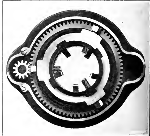
Fig. 4. Interior of Geared Die-stock shown in Fig. 2
