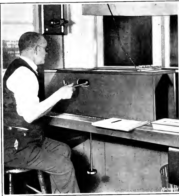
Fig. 6. View showing Case in which Comparator is enclosed when in Use to prevent Errors due to Temperature of the Observer's Body
