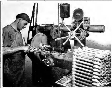
Fig. 8. Internal Grinding Operation on Large End of Connecting-rod
