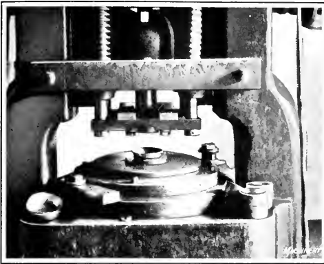
Fig. 2. Second Drawing Operation on the Aluminum Cases
