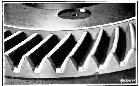
Fig. 2. Section of a Ring Bevel Gear showing Teeth which have been chamfered
