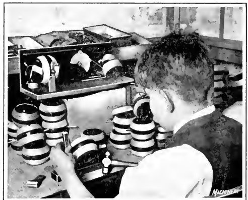
Fig. 4. Straightening the Shaft of a Variometer Rotor
