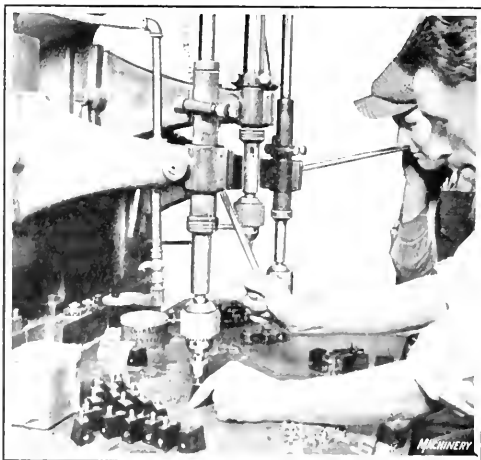
Fig. 9. Two Spindles of a Three-spindle Drilling Machine used for Spinning Operations
