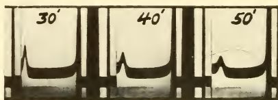
Fig. 3. Sedimentation pattern of primary glucomannan-protein (isolated from bakers' yeast cell wall) in analytical ultracentrifuge. Duration of centrifugation noted on each exposure. Note indication of low molecular weight material and apparent homogeneity of major peak.
