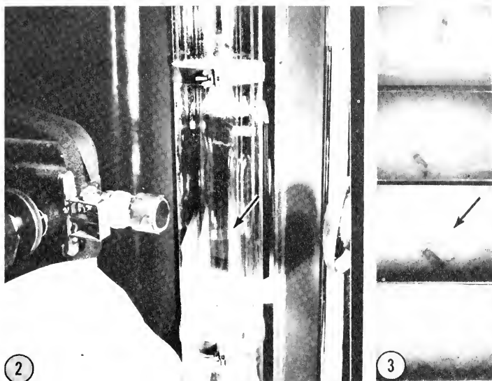
Fig. 2. Liquid helium II (arrow) in shielded Dewar at 1^{\circ} K, showing characteristic quiescent appearance. Because of the exceedingly high heat conductivity of helium II, a temperature difference between top and bottom of the liquid sufficiently great to allow the formation of vapor bubbles cannot be produced.
