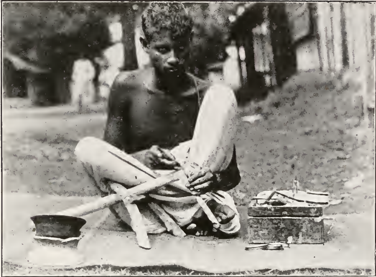
FIG. 1.—METHOD OF USING REST WHEN FINISHING OFF AN INLAID LACQUER BANGLE, DINAJPUR.
