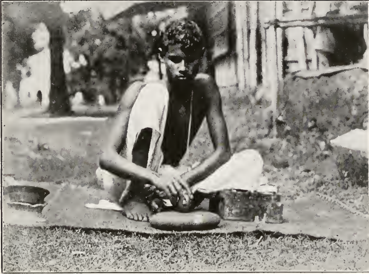
FIG. 1.—RUBBING DOWN CINNABAR TO COLOUR LACQUER RED, DINAJPUR.
