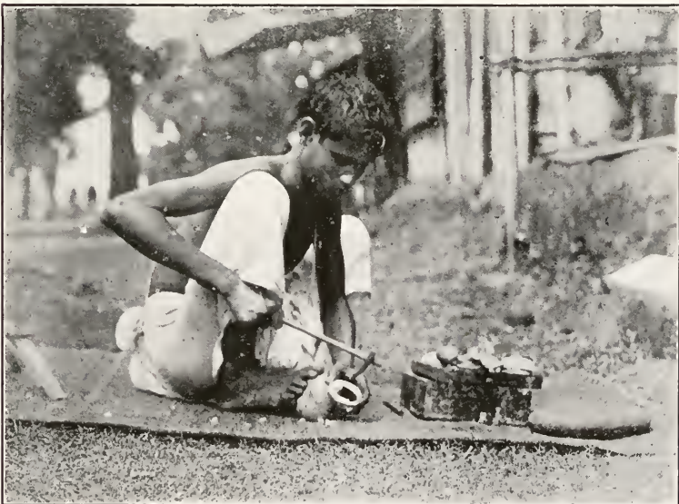
FIG. 2.—BREAKING AWAY THE REMAINS OF THE SEPTUM FROM A SAWN CHANK CIRCLE (WORKING SECTION).
