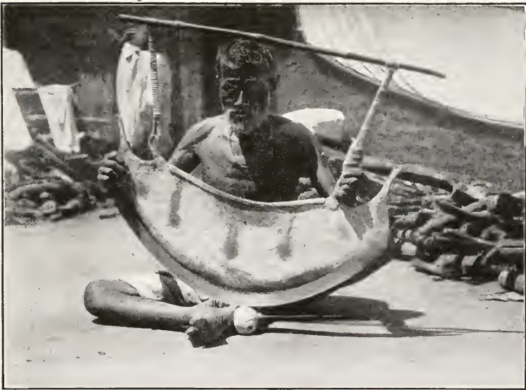
FIG. 2.—SECTIONING CHANK SHELLS IN A DACCA WORKSHOP.
