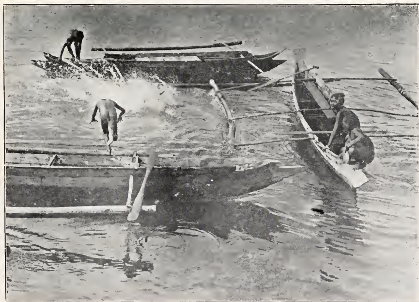
FIG. VII.—DOUBLE CANOES WITH DIRECT ATTACHMENT, JOLO, PHILIPPINE ISLANDS.
