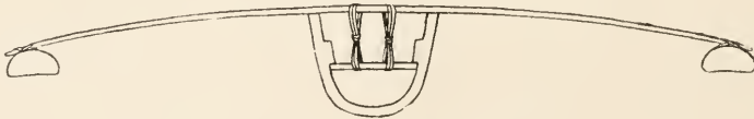
FIG. 41.—Simple form of outrigger with direct attachment; seen in section. Menado, N. Celebes.
