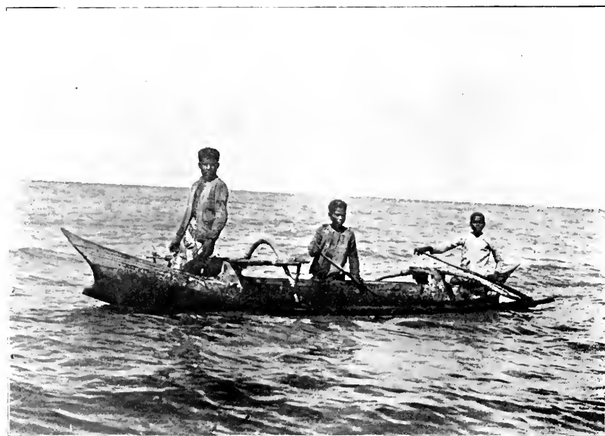
FIG. IX.—DOUBLE OUTRIGGER OF HERMAPHRODITE TYPE, MINDANAO, P.I.
