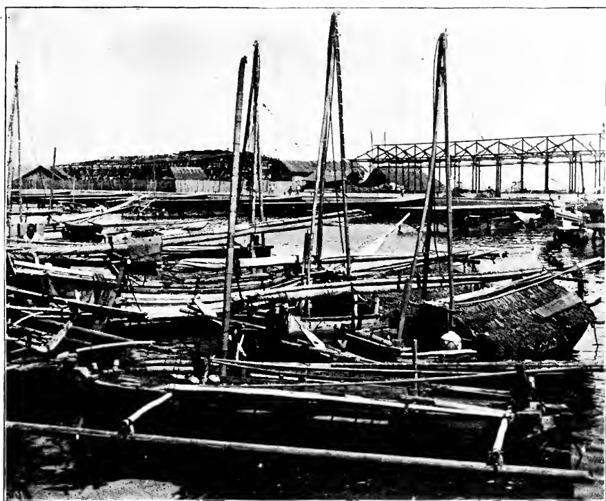
FIG. XVIII.—DOUBLE OUTRIGGER WITH SUB-DIRECT ATTACHMENT, MACASSAR.
