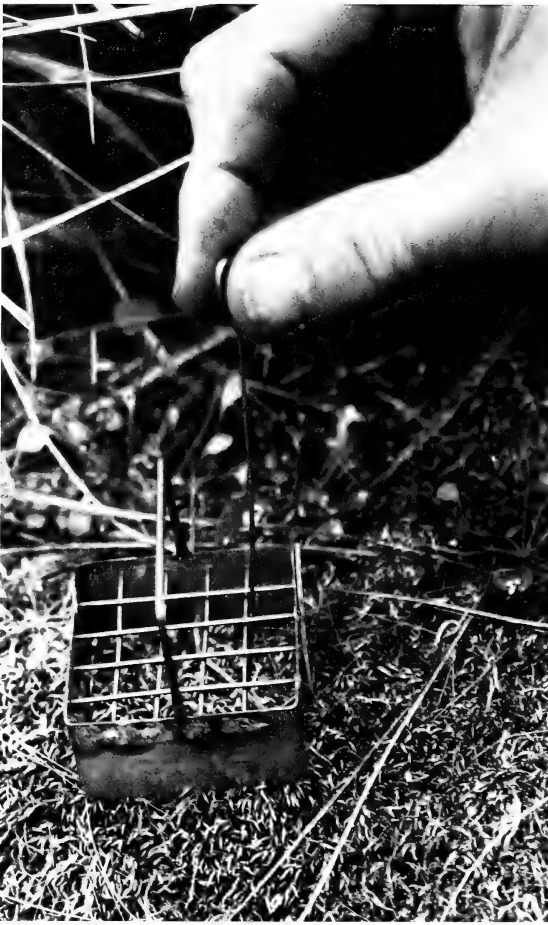
FIG. 3. Metal frame device used to extract plugs of cryptogamic crust 2 cm thick and 5 \times 5 cm in area.
