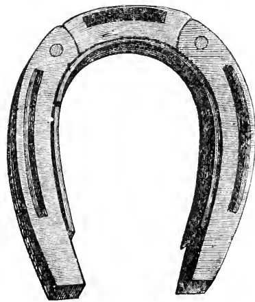
FIG. 541.—Spring Inside Shoe Riveted to Toe Part for Expanding Quarters.
