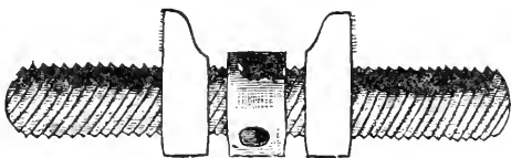
FIG. 548.—Screw for Spreading Shoe.
