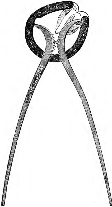
FIG. 559.—Spreaders in Position to Open the Heels.
