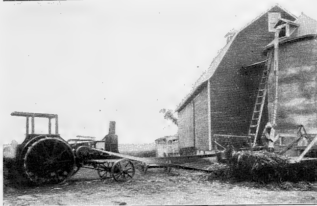
Farm tractors are efficient. Power may be applied for all purposes, both at the draw-bar and the belt.
