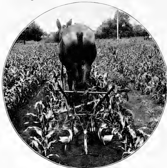
A cultivator in common use on shallow cultivated crops such as corn.
