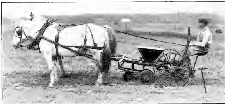
A combination Fertilizer Distributor and Planter. This implement marks off the next row, opens up the furrow for the Fertilizer, applies it, and covers it up. The furrow is again opened up, and the seed is planted, covered up, and finally the soil is pressed firmly around seeds by means of a roller.
