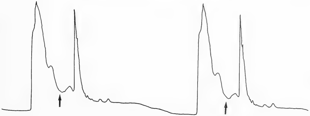
FIG. 9. HPLC spectrum of the 500 MW filtrate fraction. Two consecutive runs are shown, and the arrows indicate where the polar and non-polar fractions were separated prior to bioassay.
