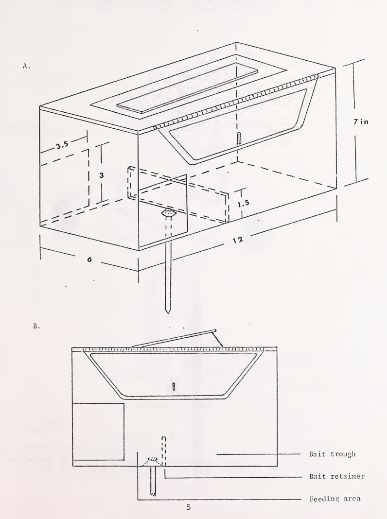
Figure 2. PVC pipe bait station. (Design by D. Sullivan, MDA)
