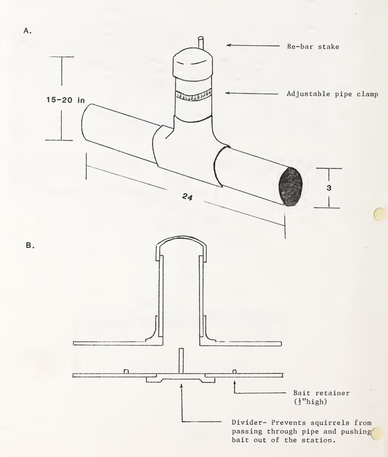
Figure 3. PVC pipe bait station (Design by S. Baril, MDA)
