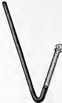
Dunbar's Fermentation Tube.
