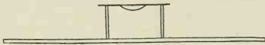
FIG. 2. Van Tieghem cell for work with hanging drop, as seen in section
