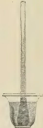
Fig. 1139. Apparatus to show osmotic action. It consists of a bladder filled with syrup, to the open end of which a tube is attached, and the whole placed in a vessel containing water.
