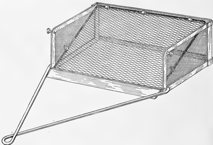
CUT 4.—Drill-dredge in position for work.
