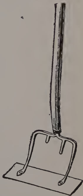
100. Home-made scarifier or scraper.
