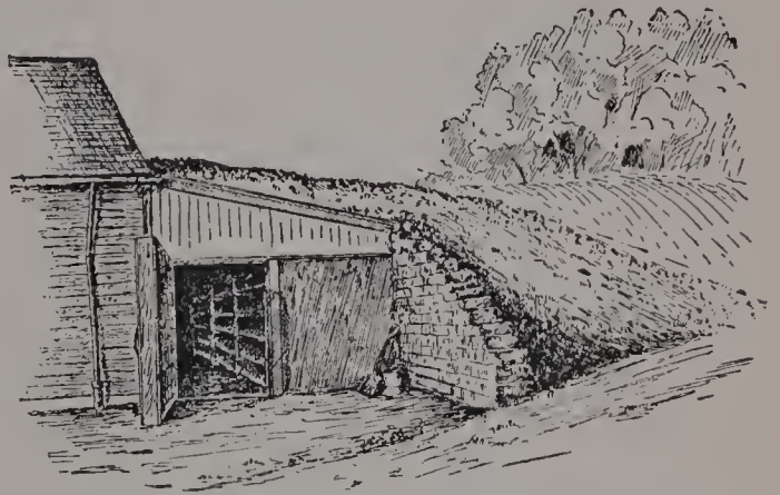
188. Lean-to fruit cellar, covered with earth. The roof should be of cement or stone slabs. Provide a ventilator.
