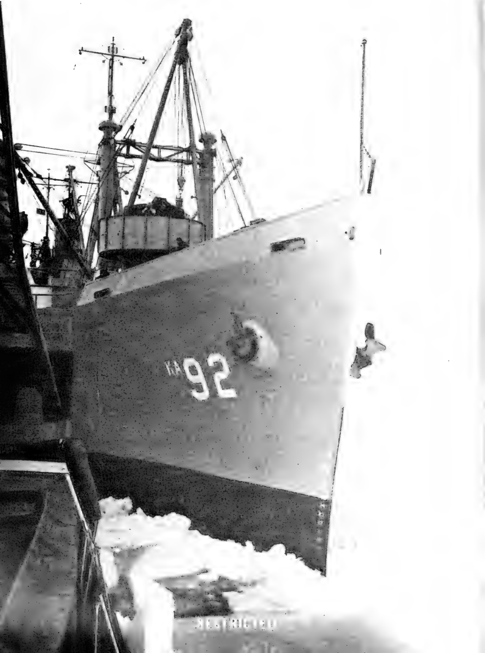
Figure 25.—U. S. C. G. Eastwind employing tactics of backing down on the bow of the U. S. S. Wyandot to break her out of ice.
