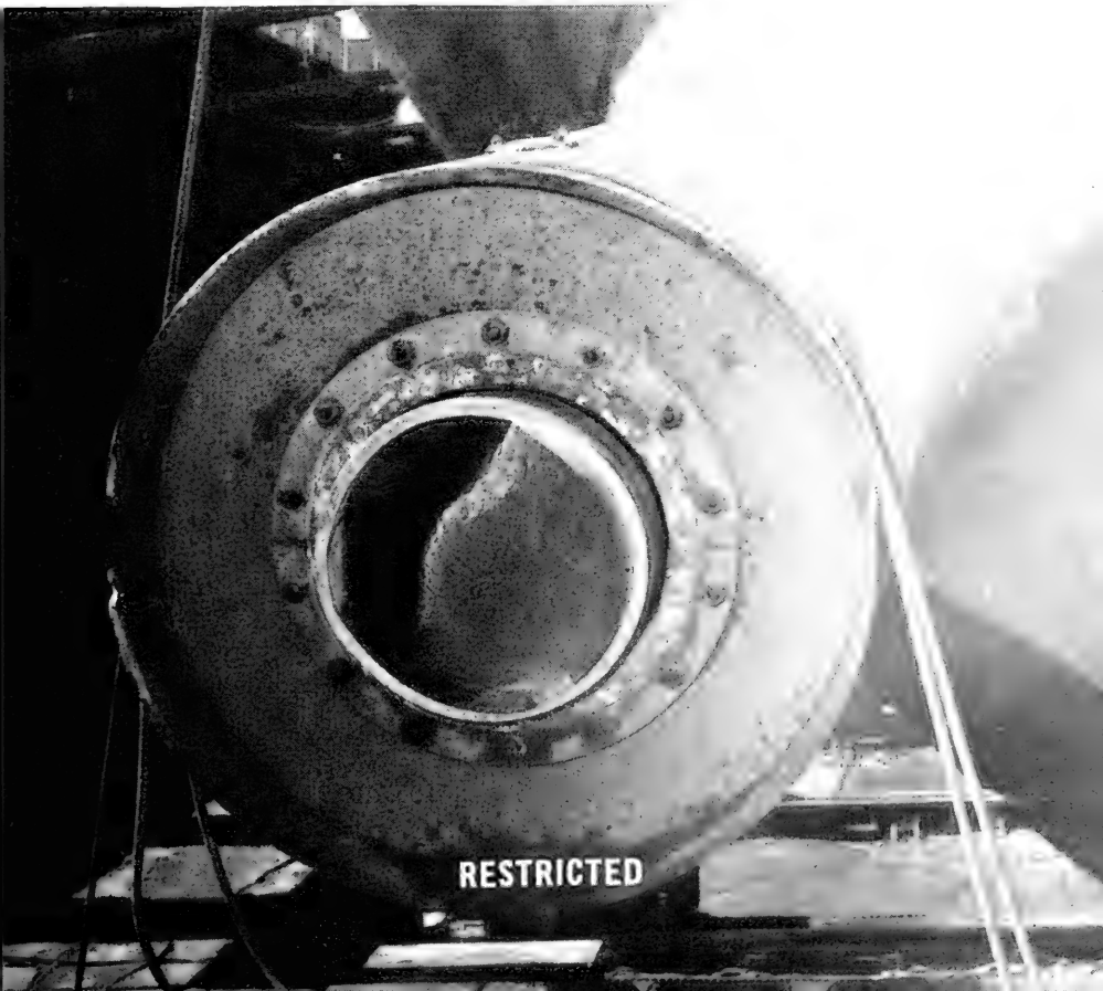
Figure 18.—U. S. S. Edisto in drydock. Port propeller and external portion of shaft were sheared off due to contact with the hard ice of the Lincoln Sea. Shaft is 18 inches in diameter.
