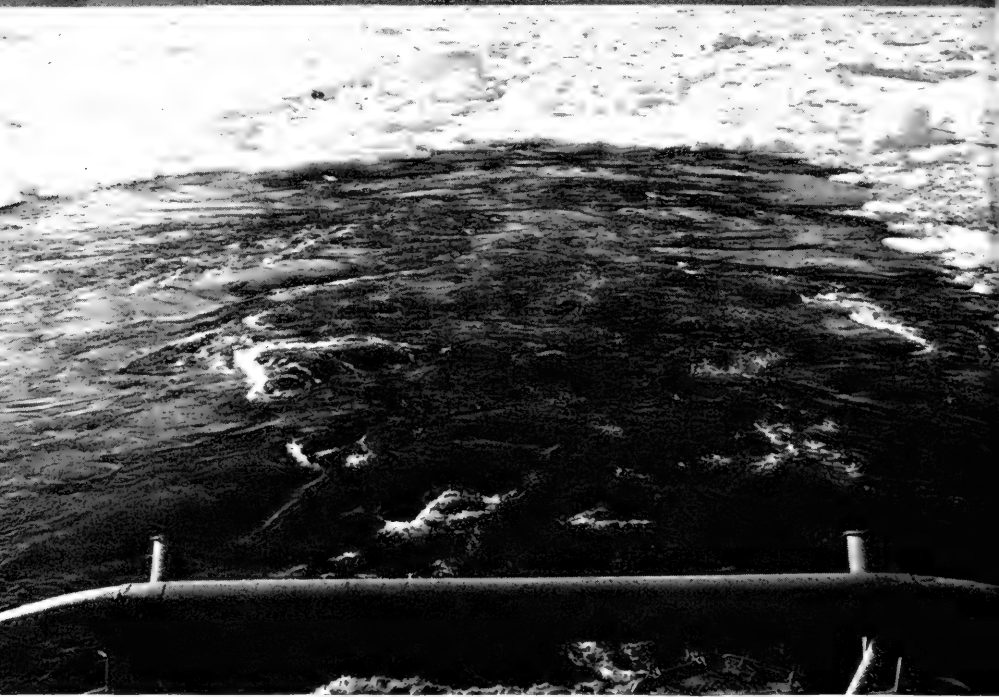
Figure 13.—Showing the effect of the propellers in keeping the stern of the icebreaker clear of ice while hove to.
