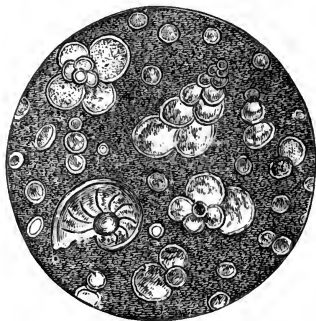
Fig. 2.—Section of Gravesend Chalk, examined by transmitted light and highly magnified. Besides the entire shells of Globigerina , Rotalia , and Textularia , numerous detached chambers of Globigerina are seen. (Original.)
