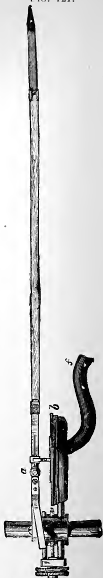
Writing Lever and Tambour.—( a ) Joint of the lever; ( b ) Air chamber; ( f ) Rubber tubing connecting it with cardiac tambour.
