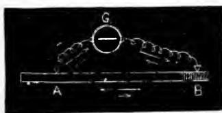
Fig. 283.—A, uninjured, B, injured, portion of nerve; G, galvanometer. The large arrows show direction of demarcation current or current of rest, the small arrows direction of negative variation or action current.
