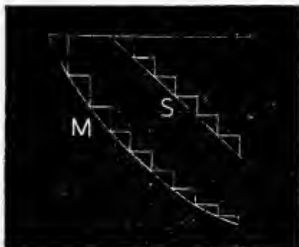
Fig. 236.—Curves of Extensibility. M, of muscle; S, of an ordinary inorganic solid.
