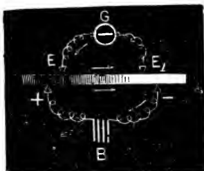
Fig. 293.—Diagram to show Distribution of 'Positive Polarization' after opening Polarizing Current. B, battery; G, galvanometer. The dark shading signifies that the excitation to which the current causing the positive deflection after the opening of the polarizing current is due is greatest in the immediate neighbourhood of the anode, and fades away in the intrapolar region. + indicates the anode, and - the kathode of the polarizing current.
