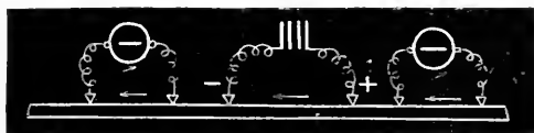
Fig. 304.—Diagram showing Direction of the Extrapolar Electrotonic Currents. + is the anode and - the kathode of the polarizing current.
