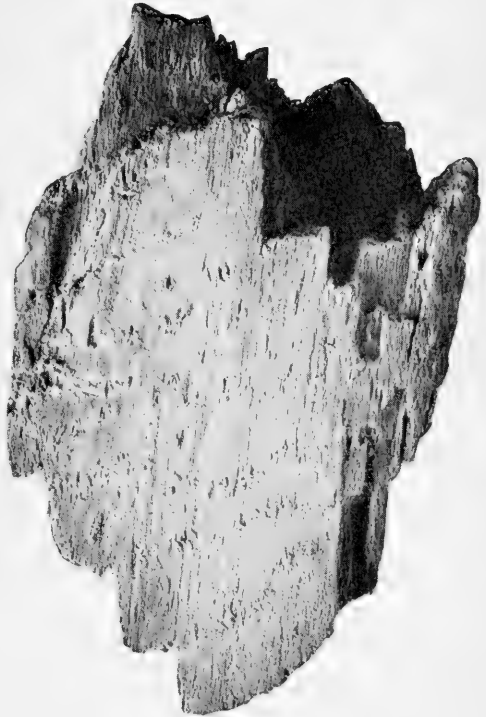
FIG. 12. — Beech wood decayed by Fomes applanatus .
