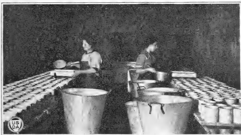
FIG. 2.—Filling the hoops, using a multiple filler, by means of which six forms are filled at the same time. (See Fig. 6.)
