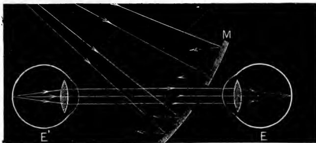
Fig. 413.—Direct Method of using the Ophthalmoscope. Light falling on the perforated concave mirror M passes into the observed eye E' ; and, both E' and the observing eye E being supposed emmetropic and unaccommodated, an erect virtual image of the illuminated retina of E' is seen by E .
