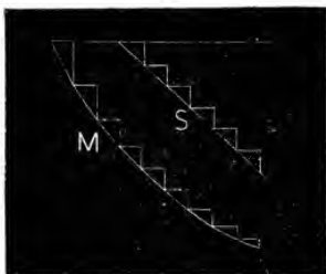
Fig. 236.—Curves of Extensibility. M, of muscle; S, of an ordinary inorganic solid.
