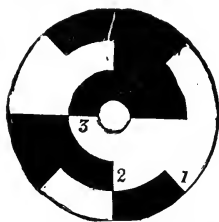
Fig. 427.—Disc for demonstrating Talbot's law.
