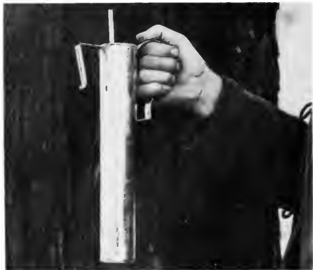
Figure 9.—Measuring the density of sap (° Brix) with a precision hydrometer calibrated in 0.1°. If the bucket contains too little sap to provide the necessary depth for the measurement, transfer the sap to a hydrometer can.
