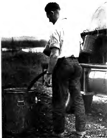
Figure 38.—Vacuum lines operated by a vacuum pump can be used to empty buckets and small containers in the woods or at the roadside.
