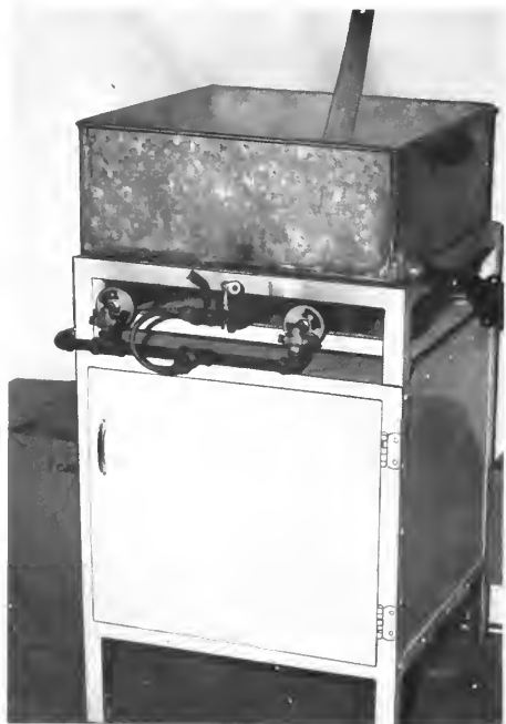
Figure 106.—Gas, whether supplied from tanks or mains, is a good source of heat for cooking maple products. The heat is easily controlled and can be stopped the instant cooking is completed. Here, sirup is being cooked for maple cream.
