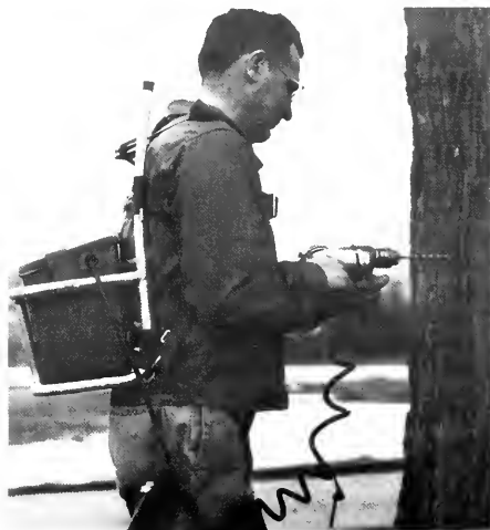
Figure 14.—An electric battery-powered tapping drill.
