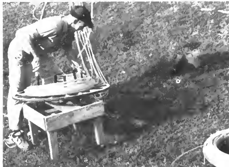
Figure 61.—The tubing is coiled on a homemade reel, tied into bundles for storage.
