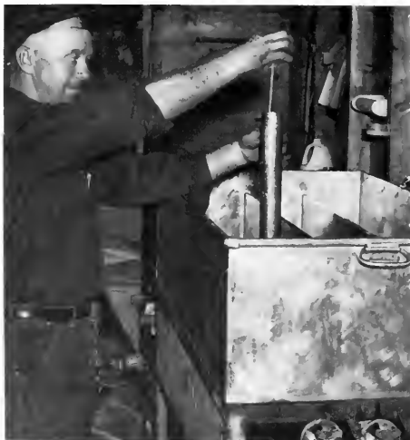
Figure 80.—The finishing pan allows complete control over the final stage of the evaporation of sap to sirup. Generally, the fuel is bottled gas.
