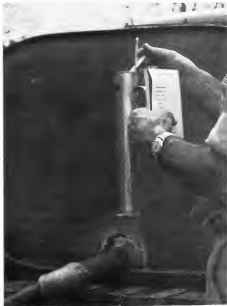
Figure 131.—A sample of sap is taken for determining its Brix value and for judging its quality. The observed Brix value, temperature, and volume of the sap are recorded for each delivery.
