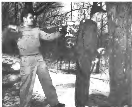
Figure 13.—A gasoline-powered portable tapping drill with flexible shaft.
