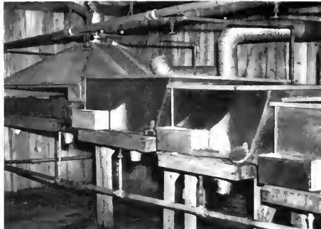
Figure 86.—This evaporator consists of several units connected in series with the partly evaporated sap moving successively to the next evaporator by means of a float control to prevent intermixing of concentrated sap with less concentrated sap.
