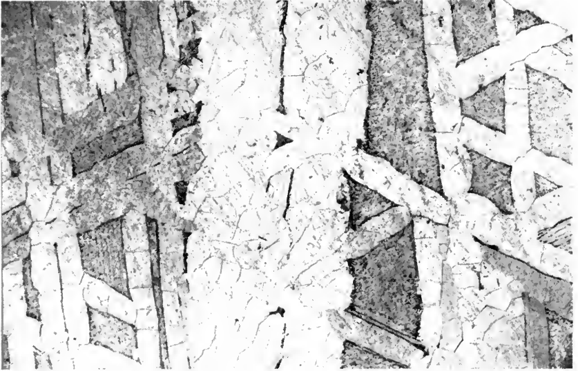
FIG. 39. At the center are two large kamacite bands. They have a swollen appearance and are not conformable with the octahedral pattern. \times 6 .
