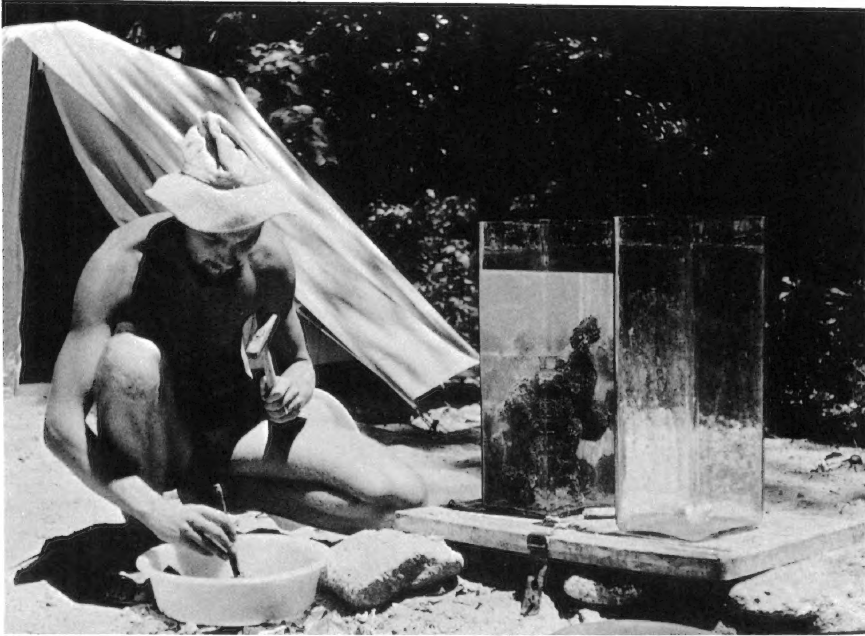
FIG. 2. Large pieces of the sample material are broken up. The substrate then is transferred to the rectangular glass jars.
