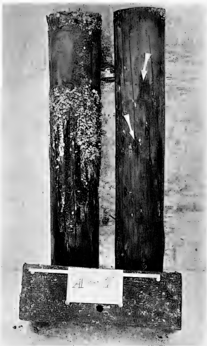
Fig. 63. Test No. A7. Douglas fir samples treated with Williams and Francois oil, photographed after 28 months' exposure. Sample at left shows heavy Limnoria attack. Sample at right shows initial Limnoria attack, as indicated by arrows. The other depressions in the surface of this sample are knots. Barnacles were scraped from this sample before photographing. Sample at bottom of photograph is a part of the creosoted frame in which the samples were held for testing; it showed no attack, the hole in the center being a bolt hole.
