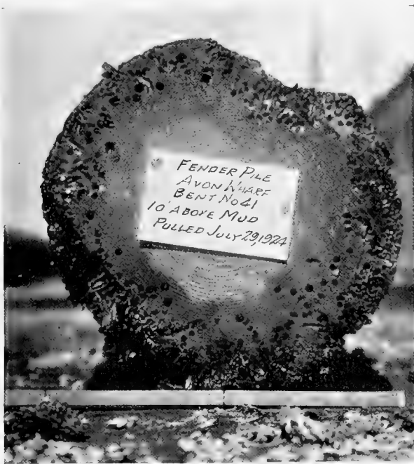
Fig. 96. Section of untreated fender pile from Avon wharf of Associated Oil Co. Pulled July 29, 1924.
