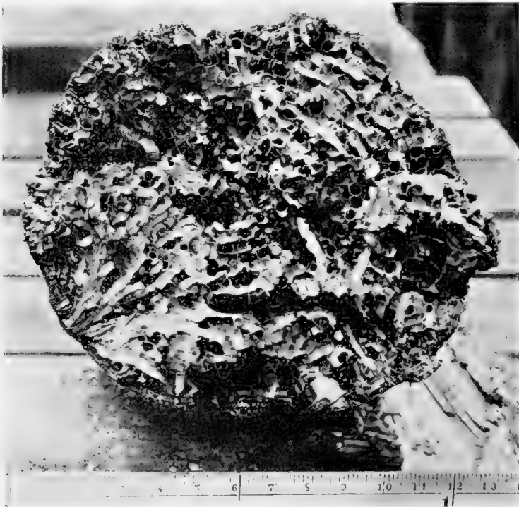
Fig. 89. Breaking point, near mud line, of pile at Oakland Mole, destroyed within 5 months by Bankia setacea .
