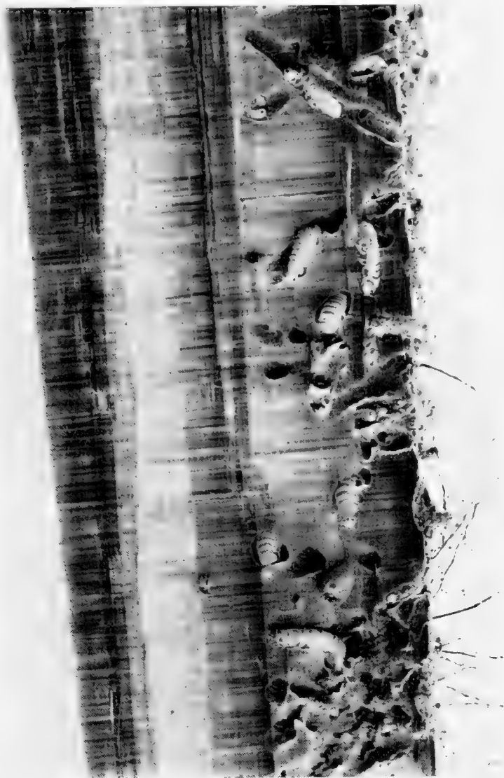
Fig. 123. Limnoria in place attacking wood. \times 5 .
