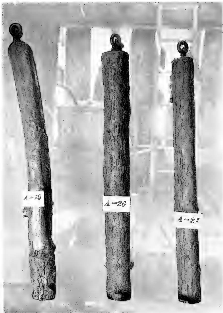
Fig. 61. Samples exposed 16\frac{1}{2} months at the Oakland Mole. No. A19. Oregon alder considerably attacked by Limnoria except in areas where bark remained on. Compare area above the white card with smooth area below, where bark was removed just before photographing. No. A20. Douglas fir sample dipped once in "Elaterite." General attack by Limnoria all over surface. No. A21. Douglas fir sample dipped twice in "Elaterite." Heavily attacked by Limnoria . Diameter considerably reduced.
