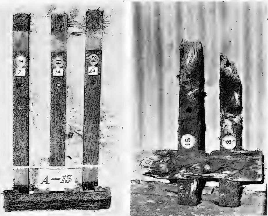
Fig. 64. (1) Test No. A13. Pine samples treated with paraffine after the method of Dr. Paul Bartsch. Photographed after 17 months' exposure. No. 7 is treated with paraffin only, No. 14 with paraffine and copper iodide, and No. 24 with paraffine and arsenious iodide. All heavily attacked by Limnoria . Sample at bottom is untreated control. (2) Test No. B18. Samples No. 8 and No. 15, treated as were No. 7 and No. 14 of test A13. Photographed July 19, 1924, after 31 months' exposure. Attacked by Limnoria , Bankia and Teredo .
