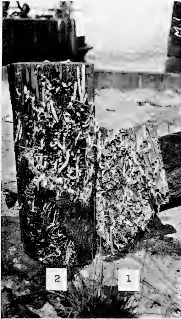
Fig. 116. Pile from Seattle, driven December, 1922, pulled June, 1924. Entirely destroyed at mud line by Bankia setacea .
