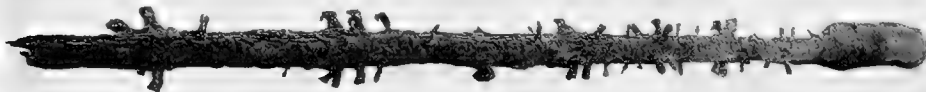
Fig. 30. Green test pile driven at west end of Alameda Distributing Station Dock in December, 1920. Pulled November 27, 1923. Depth of water at high tide 25 feet. Original dimensions of pile 40 feet long, 14-inch butt, 8-inch tip.
