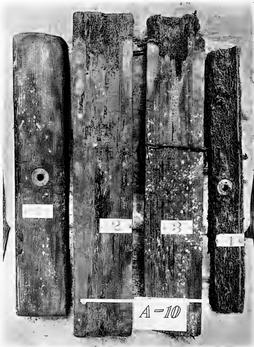
Fig. 65. Test No. A10. Douglas fir samples treated by Arent Laboratories with benzol antimony trichloride (No. 2) and creosote antimony trichloride (No. 3), after 28 months' exposure. Both heavily attacked by Limnoria . No. 1 is a portion of the creosoted frame, and No. 4 an untreated control.
